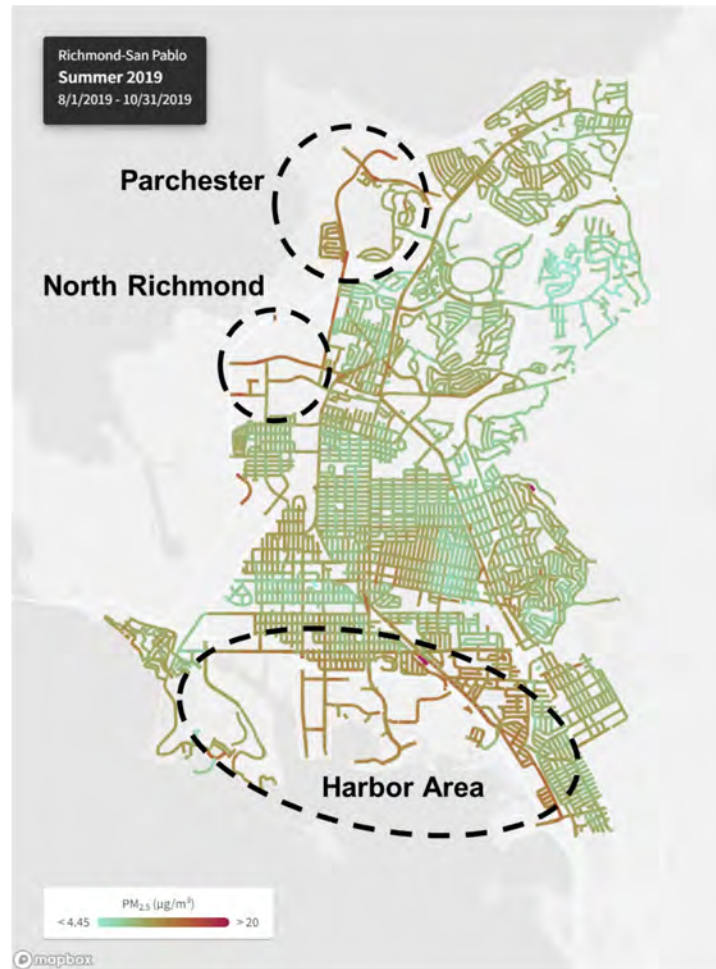
Figure 5-10. Screenshot from Aclima’s Richmond-San Pablo PM 2.5 Report, annotated with areas where higher levels of PM 2.5 were found. Air monitoring for this specific project was conducted from August to October 2019.
