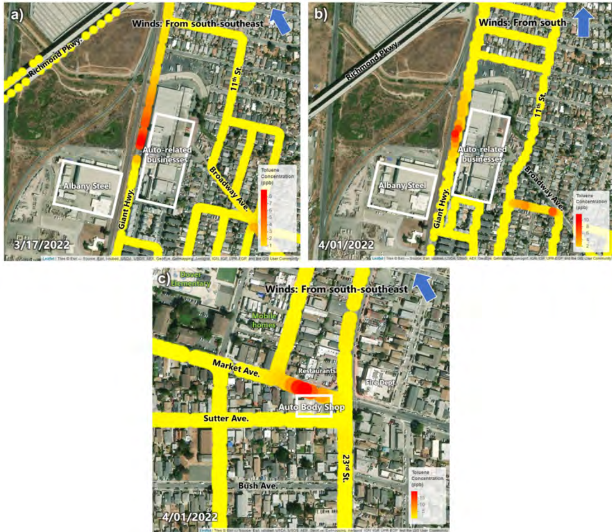
Figure 11. Relatively higher levels of toluene were measured near and downwind of autobody shops along a) Giant Hwy. on 3/17/2022, b) Giant Hwy. on 4/1/2022, and c) Market Ave. on 4/1/2022.
