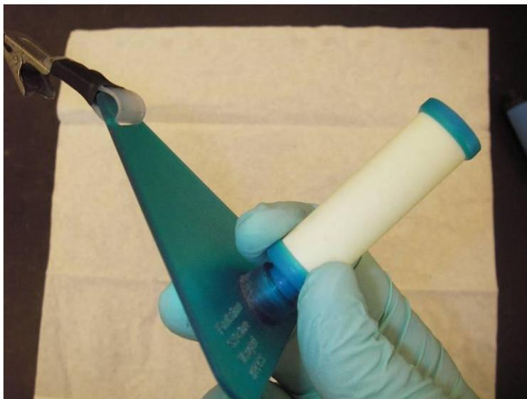
Assembly of the Radiello Passive Sampler is now complete. Use the metal clip to attach the sampler to clothing for personal exposure monitoring or to another object for ambient
