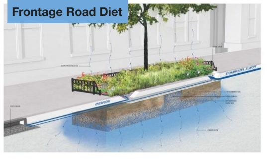
A series of stepped bioswales to absorb water.
