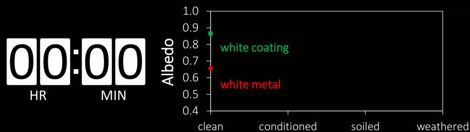
LBNL laboratory aging method quickly predicts 3-year-aged roof albedo, thermal emittance
