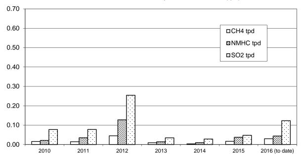
The Rodeo Refinery installed and has utilized a Flare Gas Recovery Compressor since the mid-70's. Historic practices emphasized flare minimization. Some of the recent flaring reductions have occurred due to improved monitoring and tracking of flare volumes as well as attributing causes to all flaring as required by BAAQMD 12-11 and 12-12 and internal policies for incident investigation. Other efforts to minimize flare emissions have occurred through communication and improved awareness.
