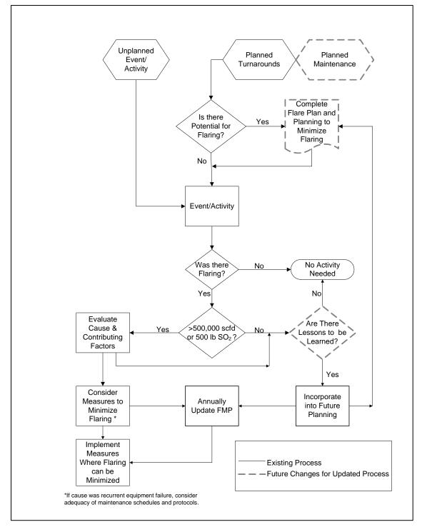
Figure 5-1, Flare Planning Process Flowchart
