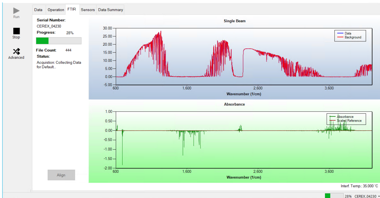
Figure 2. Screenshot showing the FTIR tab of the CMS software. Note that the Align and Run buttons are grayed out because the instrument is in run mode.
