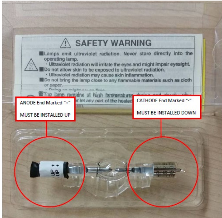
Figure 8. The ANODE end of the UV Source is marked (+). The CATHODE end of the UV Source is marked (-).
