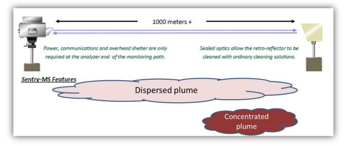
**Figure 1**. Basic premise for open-path instrument operation. Image from CEREX Sentry-MS monitoring brochure.
