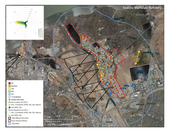
**Figure 10.** Proposed open-path monitoring sites for the Tesoro Martinez Refinery. Four proposed paths are identified, labeled 1n-1s, 2e-2w, 3n-3s, and 4n-4s. The annual wind rose is shown in the top left.
