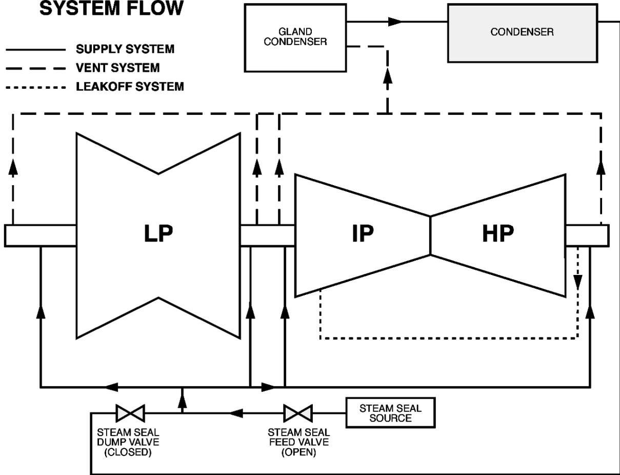
Figure 5. Steam Flow at Startup: D Series
