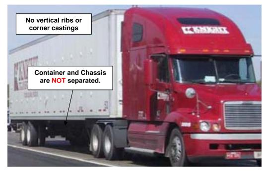
Figure 10: Examples of Non-Port Container Trucks without Vertical Ribbing
