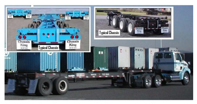
Figure 7. Chassis Truck
