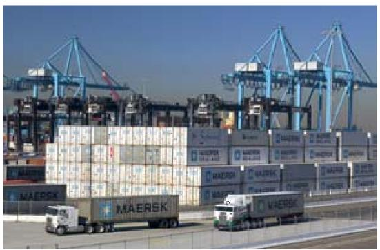
Container trucks without the typical ribbing and corner castings were not counted as Port related vehicles, but were counted as non-drayage trucks based on the number of axles. Container trailers for non-Port activities are typically 53 feet long with the container built on the chassis as a single unit (see Figure 10). The Port trucks are easily differentiated from the non-drayage trucks based on their size and characteristic vertical ribbing and corner castings on the container.
