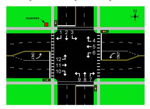
Figure 5. Vehicle Turning Movement Designations
