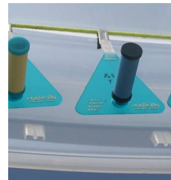
Radiello passive samplers for VOC, aldehydes and H 2 S (size of a roll of pennies)
