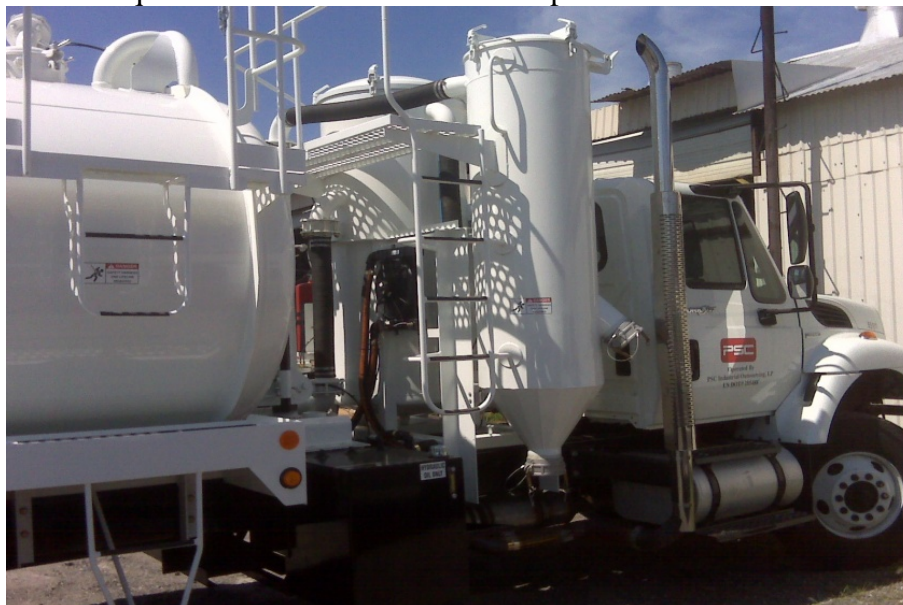
Figure 10 Vacuum Truck Containing a Combination of a Liquid Scrubber and Carbon Adsorption Control Device
