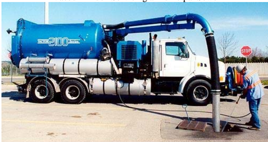
Figure 2 Vacuum Truck Servicing a Municipal Sewer
