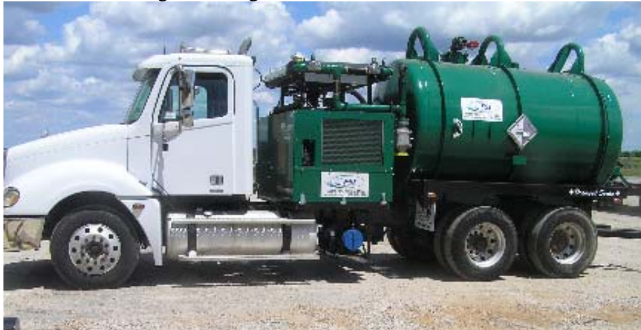
Figure 7 Vacuum Truck with a Combination I.C. Engine-Refrigerated Condenser Control Device
