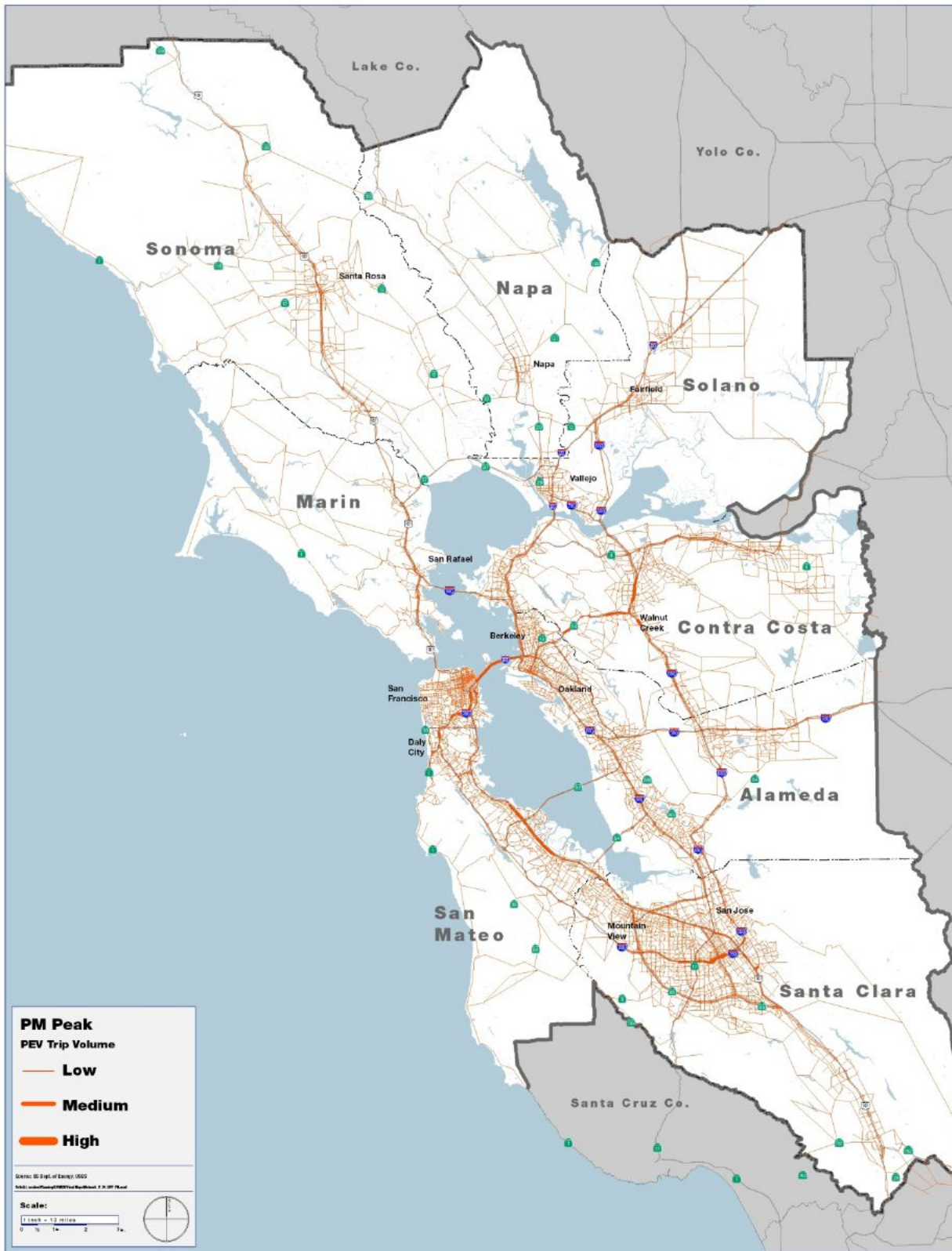
Figure 24. Heavy Volume Corridors during evening peak traffic: Siting for DC fast charging
