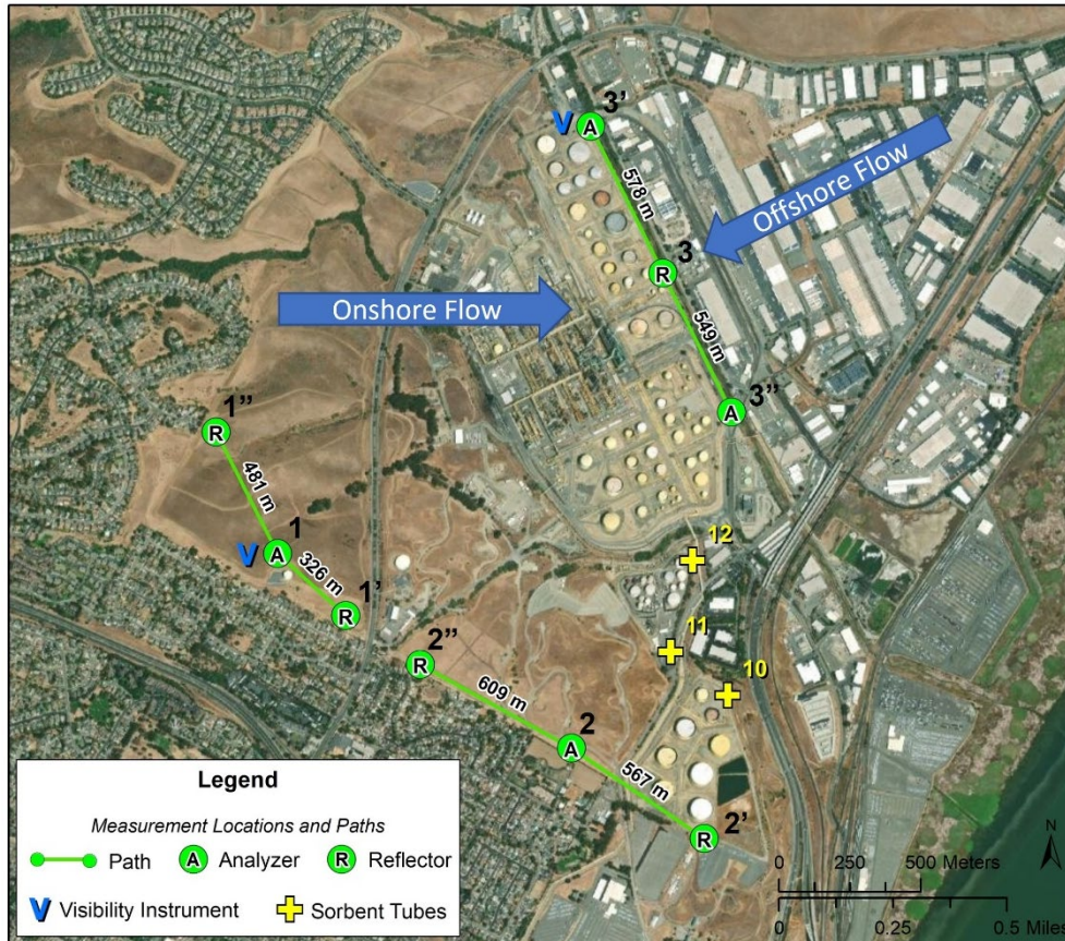
Figure 2. Open-path monitoring network for Valero’s Benicia Refinery. Each path is numbered and contains segments that are labeled with the path number and a prime (') or double prime (") symbol. Main wind flow directions are also shown.
