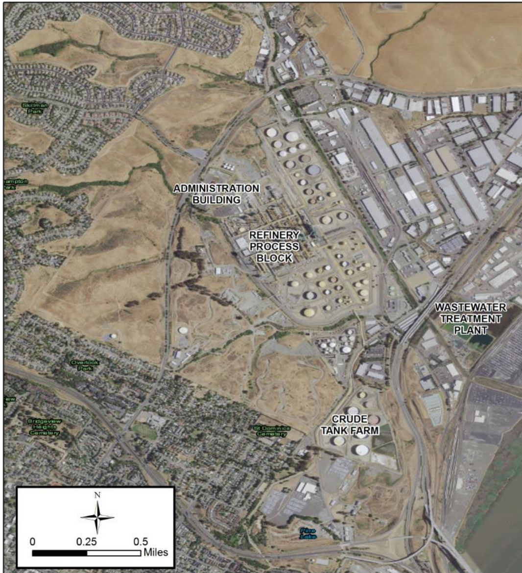
Figure 4. Layout of the Valero Benicia Refinery (Source: Valero Improvement Project Environmental Impact Report, June 2008).
