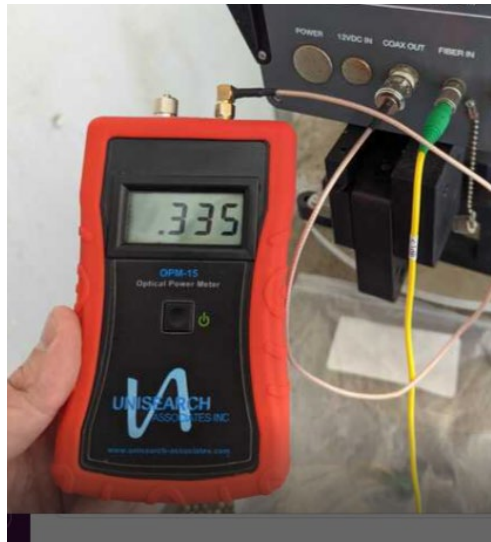
Figure 5. Measuring laser power with the OPM-15 meter provided.
