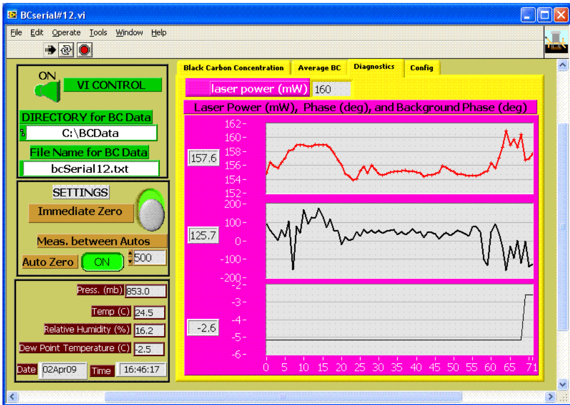
Diagnostics tab of photoacoustic instrument LabView program. Top graph shows laser power during warmup (not stabilized yet).
