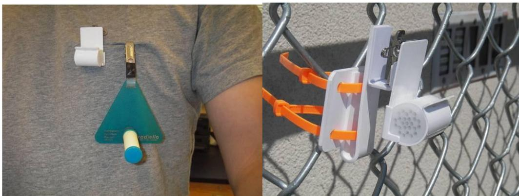
The *Mounting Bracket* can be easily attached to objects such as fences and poles with zip ties. If sampling outdoors, the *Opaque Vial* should be used as a shelter. It can easily be slipped over the
