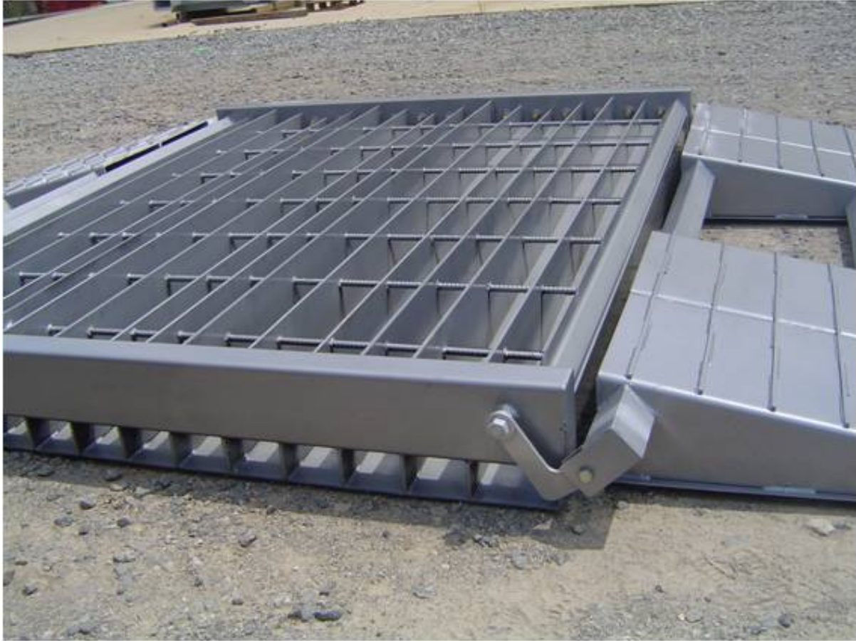
Figure II-3: Grizzly used to control Trackout
