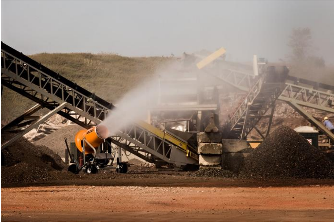
Figure II-4: Use water fog or mist to control dust during active handling operations.
