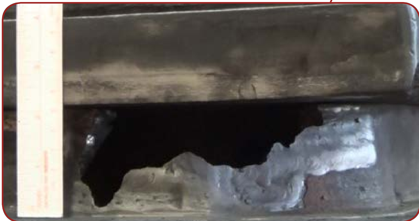
Figure 3. The Husky Superior FCCU SCSV post-incident. The top picture shows the entire valve assembly and the bottom picture shows the eroded orifice port.
