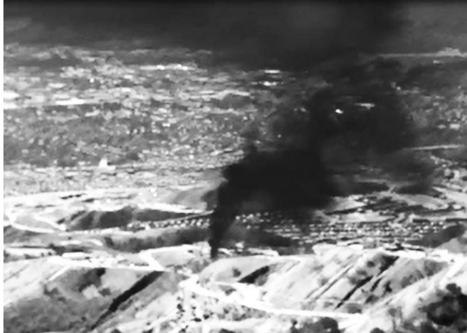
Figure 1- Infrared image showing a methane emissions plume from the Aliso Canyon natural gas storage facility 15
