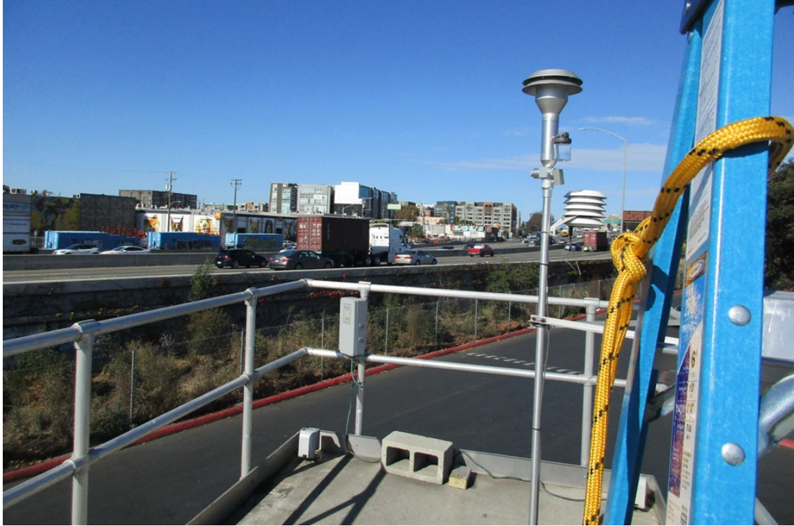
Figure 5-22: Locations of the Air District's near-road air monitoring sites (top) and photo of the probe at the Oakland – Laney near-road air monitoring site near I-880 (bottom). 151
