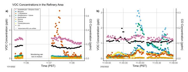
*Figure 14.* Time-series of VOC and CO concentrations measured a) along Ohio Avenue on 1/31/2022 and b) near the Chevron Refinery on 2/02/2022.
