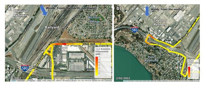
*Figure 13.* Map views of measured a) 1,3-butadiene concentrations along Ohio Avenue on 1/31/2022 and b) toluene concentrations near the Chevron Refinery on 2/02/2022.
