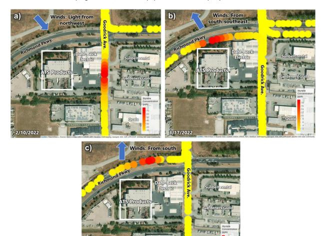
*Figure 9.* Map views of styrene concentrations measured along Richmond Parkway and Goodrick Avenue near a plastics ductwork fabrication facility on a) 2/10/2022, b) 3/17/2022, and c) 4/01/2022.
