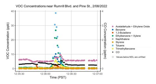
Figure 12. Time-series of VOC and CO concentrations measured near a gas station along Pine Avenue, 2/08/2022.
