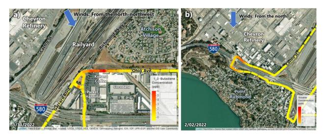
**Figure 13.** Map views of measured a) 1,3-butadiene concentrations along Ohio Avenue on 1/31/2022 and b) toluene concentrations near the Chevron Refinery on 2/02/2022.
