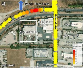
**Figure 9.** Map views of styrene concentrations measured along Richmond Parkway and Goodrick Avenue near a plastics ductwork fabrication facility on a) 2/10/2022, b) 3/17/2022, and c) 4/01/2022.
