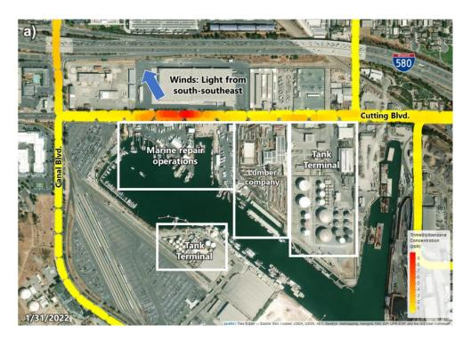
**Figure 7a.** Map view of trimethylbenzene concentrations measured along Cutting Boulevard near tank terminals and marine operations on 1/31/2022.
