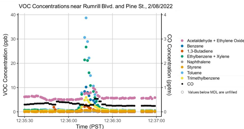
**Figure 12.** Time-series of VOC and CO concentrations measured near a gas station along Pine Avenue, 2/08/2022.
