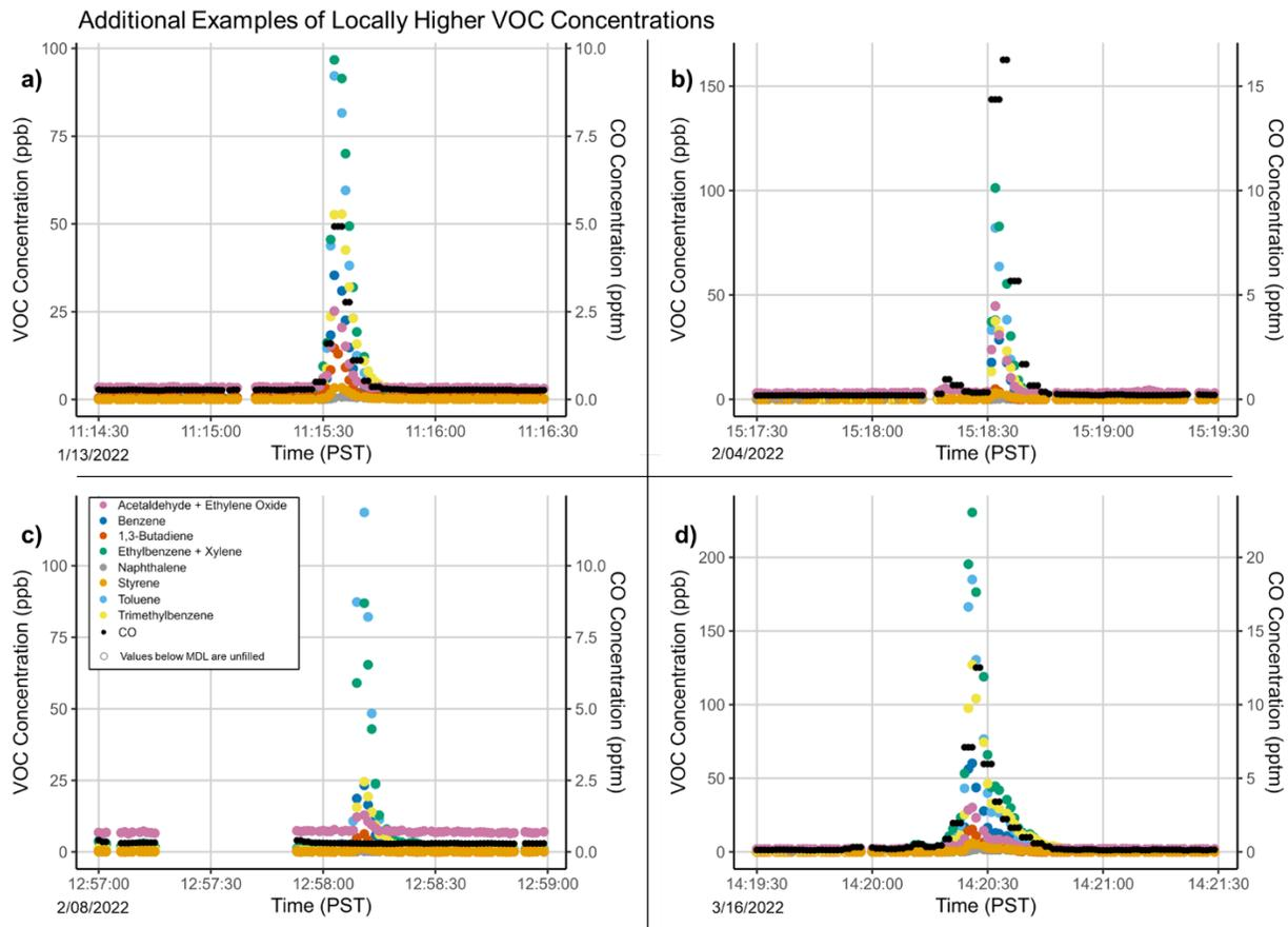
**Figure 22.** Time-series of VOC and CO concentrations measured during additional examples of peaks in VOCs, measured along a) Sanford Avenue on 1/13/2022, b) 25<sup>th</sup> Street on 2/04/2022, c) Rheem Avenue on 2/08/2022, and d) Cutting Boulevard on 3/16/2022.
