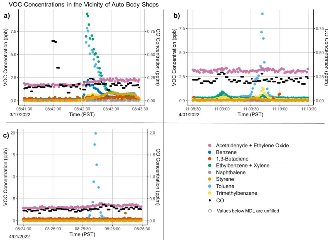
**Figure 16.** Time-series of VOC and CO concentrations measured in the vicinity of auto body shops along a) Giant Highway on 3/17/2022, b) Giant Highway on 4/01/2022, and c) Market Avenue on 4/01/2022.
