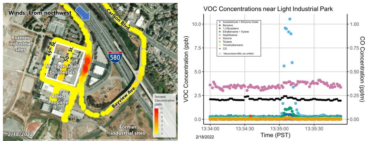
**Figure 21.** Map view of measured toluene concentrations (left) and time-series of measured VOC and CO concentrations (right) near a light industrial park off I-580, 2/18/2022.
