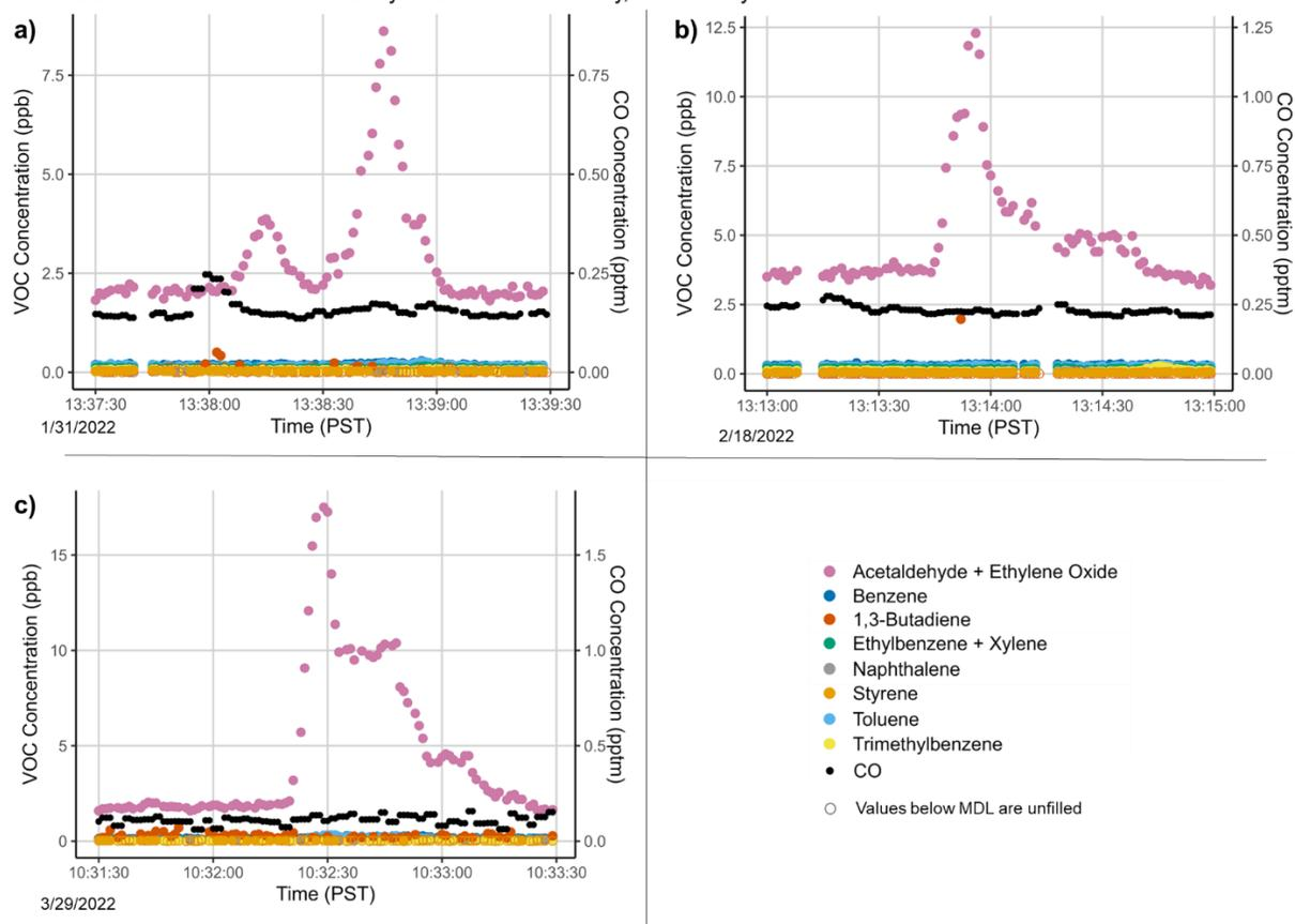
**Figure 18.** Time-series of VOC and CO concentrations measured in the vicinity of a commercial bakery in Marina Bay on a) 1/31/2022, b) 2/18/2022, and c) 3/29/2022.
