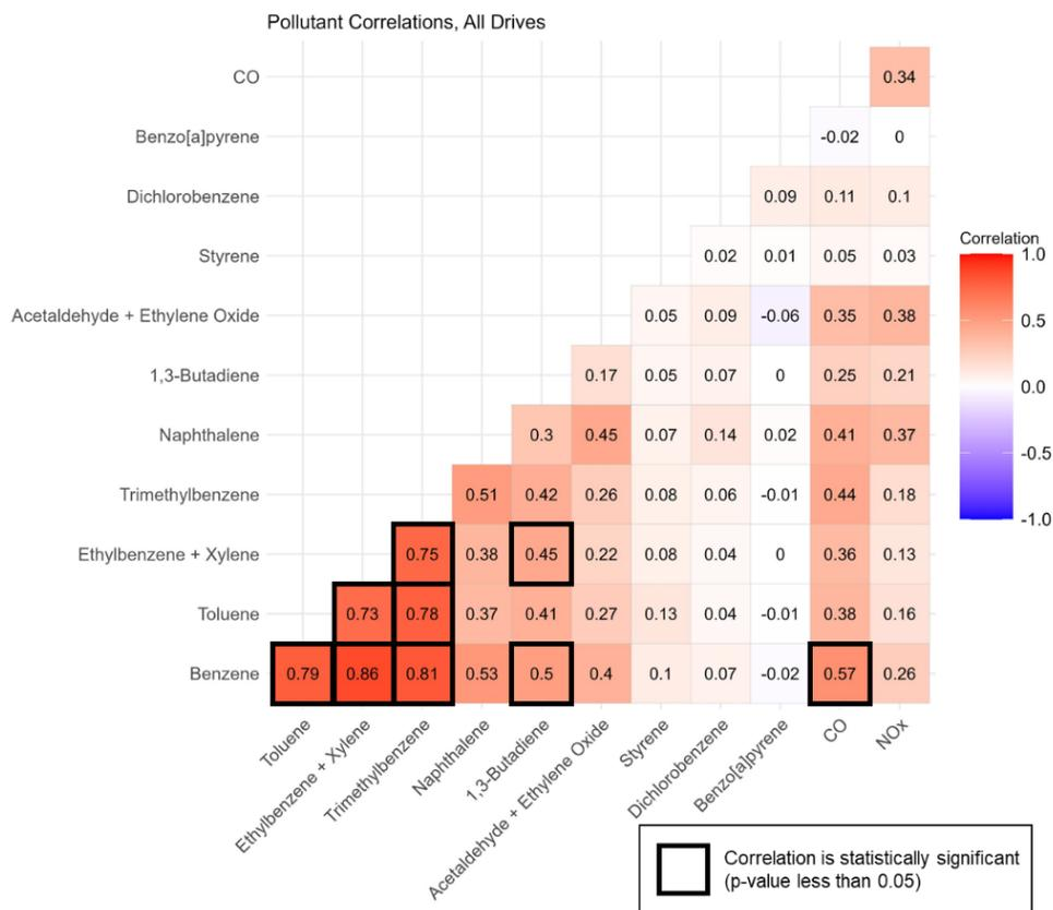
**Figure 4.** Correlation matrix for target VOCs, CO, and NO<sub>x</sub> across all drive days. Darker red shading indicates a higher positive correlation. Bolded squares indicate that the correlation is statistically significant.
