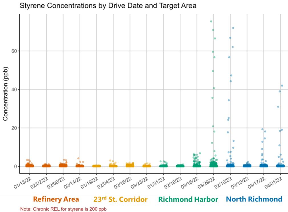
**Figure A-10.** Instantaneous (1-second) styrene concentrations by drive date and target area. The chronic REL for styrene is provided for reference but note that the chronic REL is based on annual exposures.
