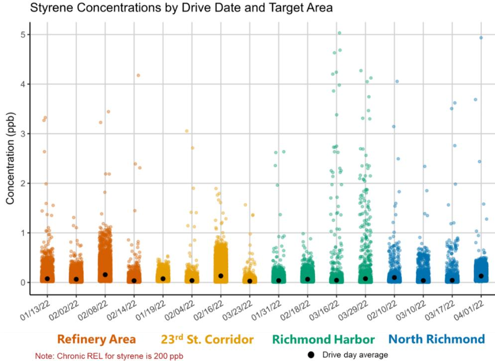
**Figure A-11.** Similar to Figure A-10, instantaneous (1-second) styrene concentrations by drive date and target area, but zoomed in on concentrations below 5 ppb to better visualize variability in concentrations across drive days. The chronic REL for styrene is provided for reference but note that the chronic REL is based on annual exposures.
