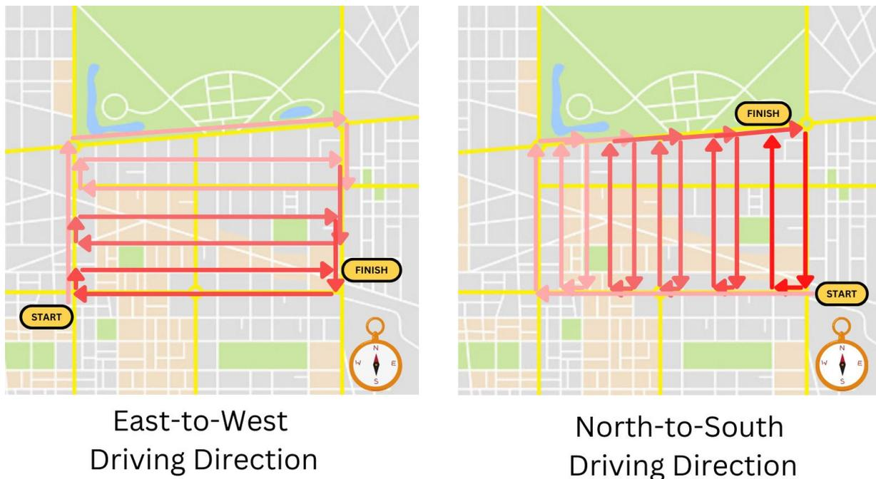
**Figure 3.** Right-Hand Box Method. The lighter colored arrows indicate earlier in the drive and the darker arrows indicate later in the drive.
