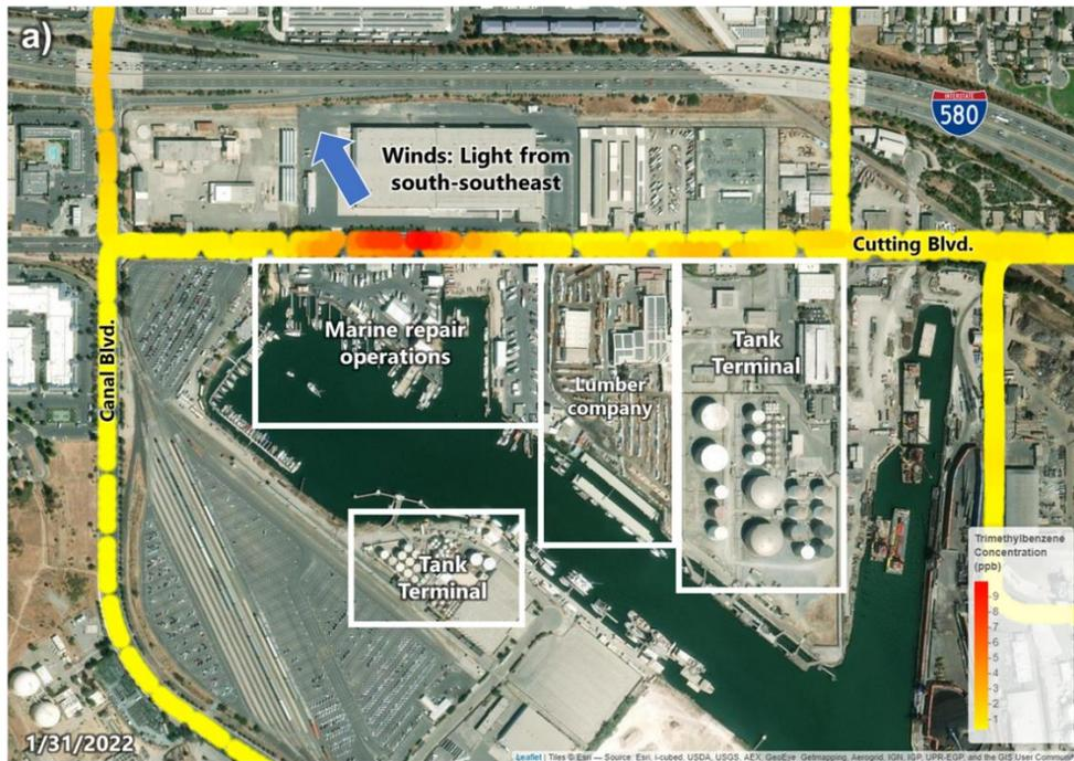
**Figure 7a.** Map view of trimethylbenzene concentrations measured along Cutting Boulevard near tank terminals and marine operations on 1/31/2022.
