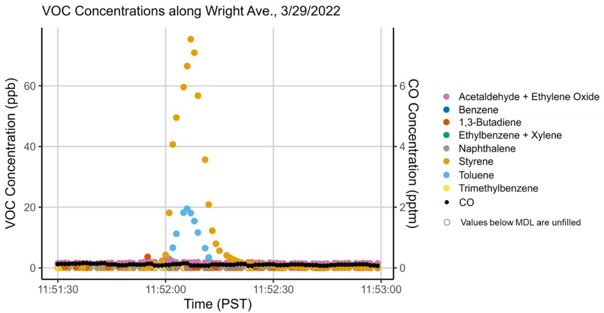
Figure 6. Time-series of VOC and CO concentrations measured near a tank terminal along Wright Avenue, 3/29/2022.
