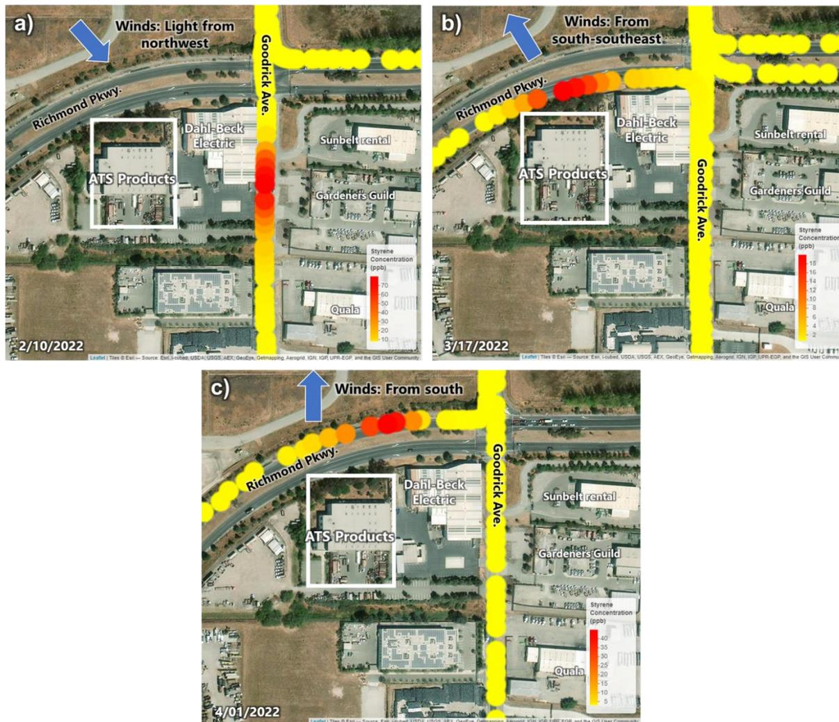
**Figure 9.** Map views of styrene concentrations measured along Richmond Parkway and Goodrick Avenue near a plastics ductwork fabrication facility on a) 2/10/2022, b) 3/17/2022, and c) 4/01/2022.
