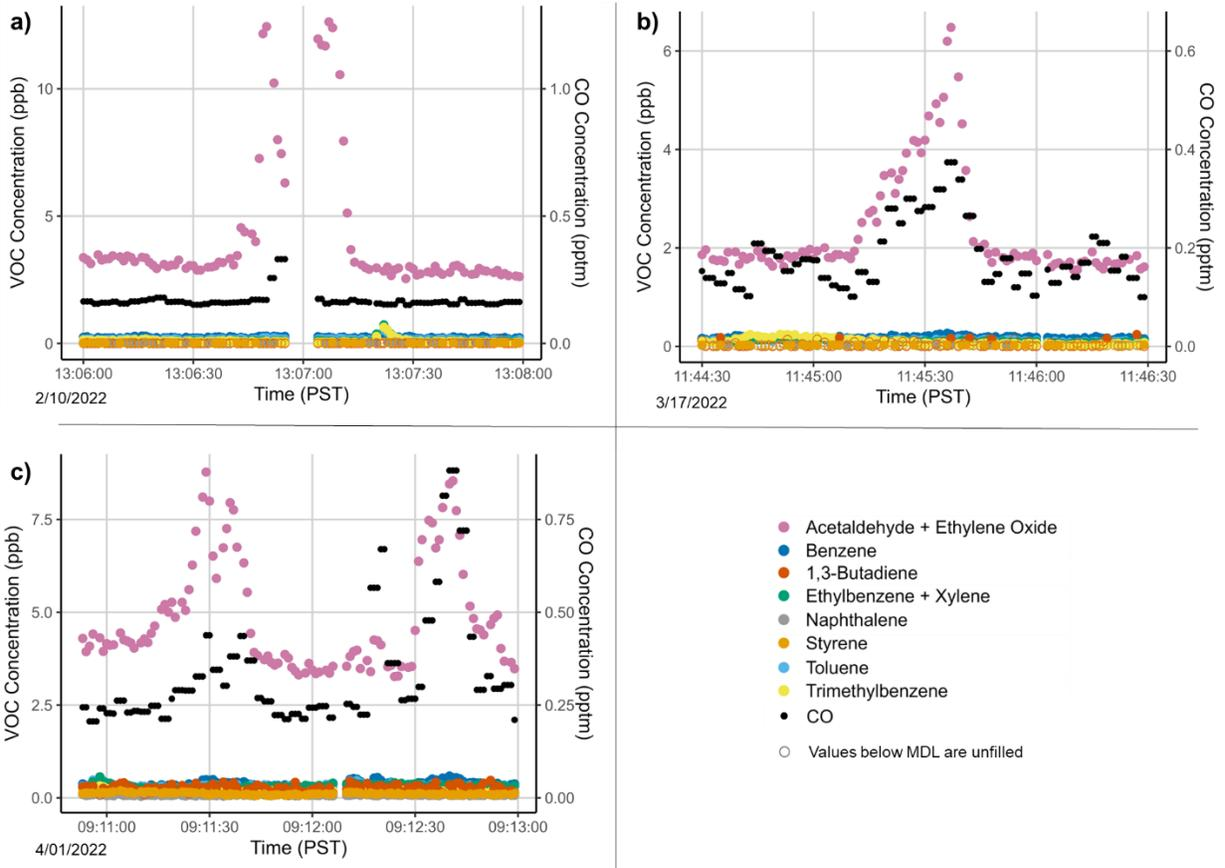
**Figure 20.** Time-series of VOC and CO concentrations measured in the vicinity of a commercial bakery near North Richmond on a) 2/10/2022, b) 3/17/2022, and c) 4/01/2022.
