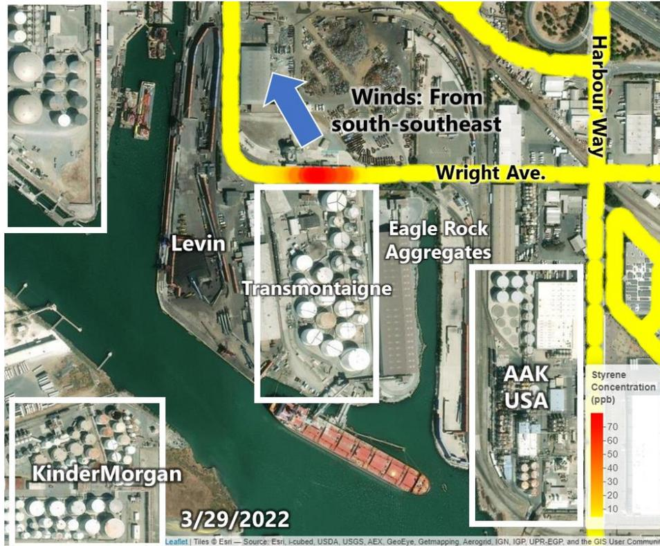
Figure 5. Map view of styrene concentrations measured near a tank terminal along Wright Avenue, 3/29/2022.
