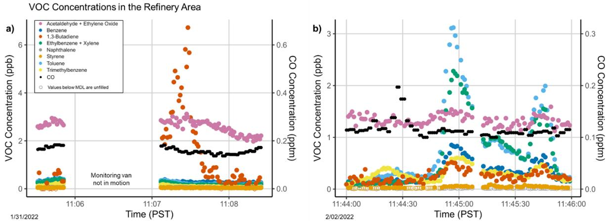
**Figure 14.** Time-series of VOC and CO concentrations measured a) along Ohio Avenue on 1/31/2022 and b) near the Chevron Refinery on 2/02/2022.
