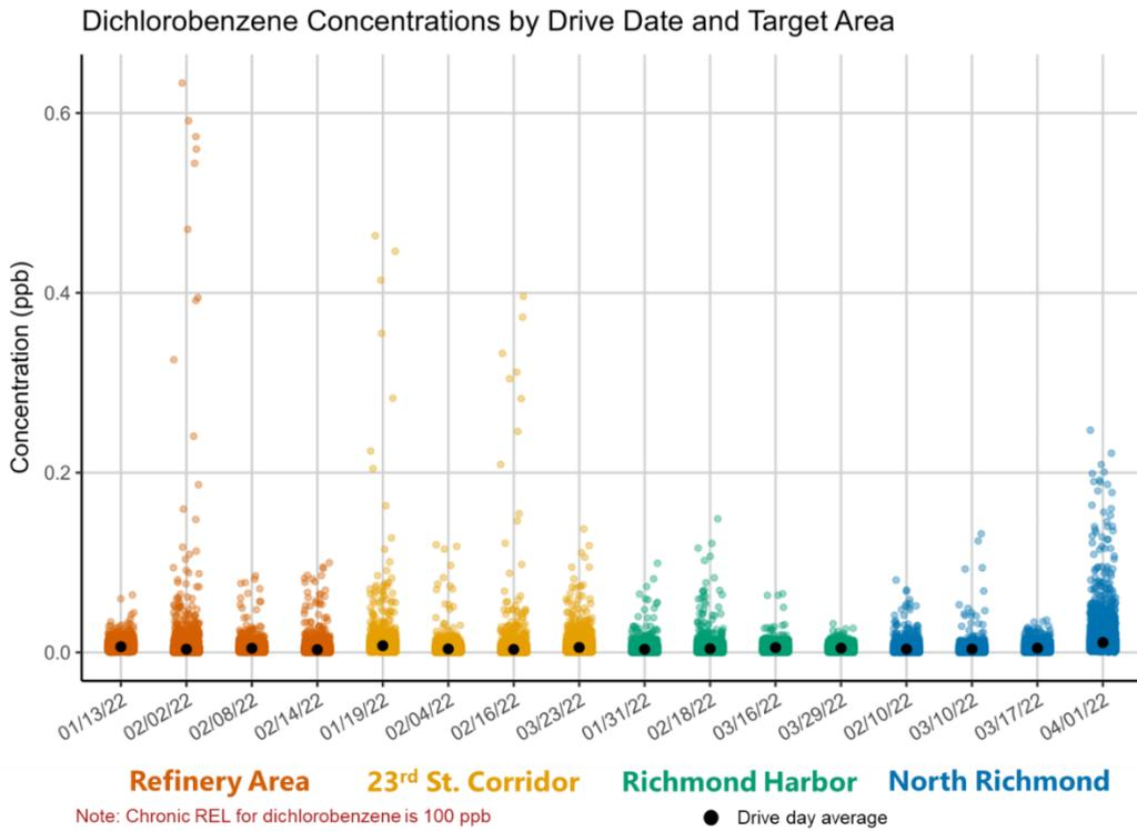
**Figure A-6.** Instantaneous (1-second) dichlorobenzene concentrations by drive date and target area.
