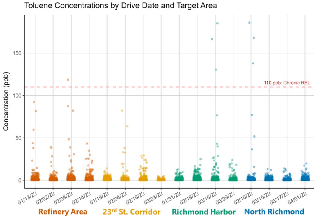
**Figure A-12.** Instantaneous (1-second) toluene concentrations by drive date and target area. The chronic REL for toluene is provided for reference but note that the chronic REL is based on annual exposures.
