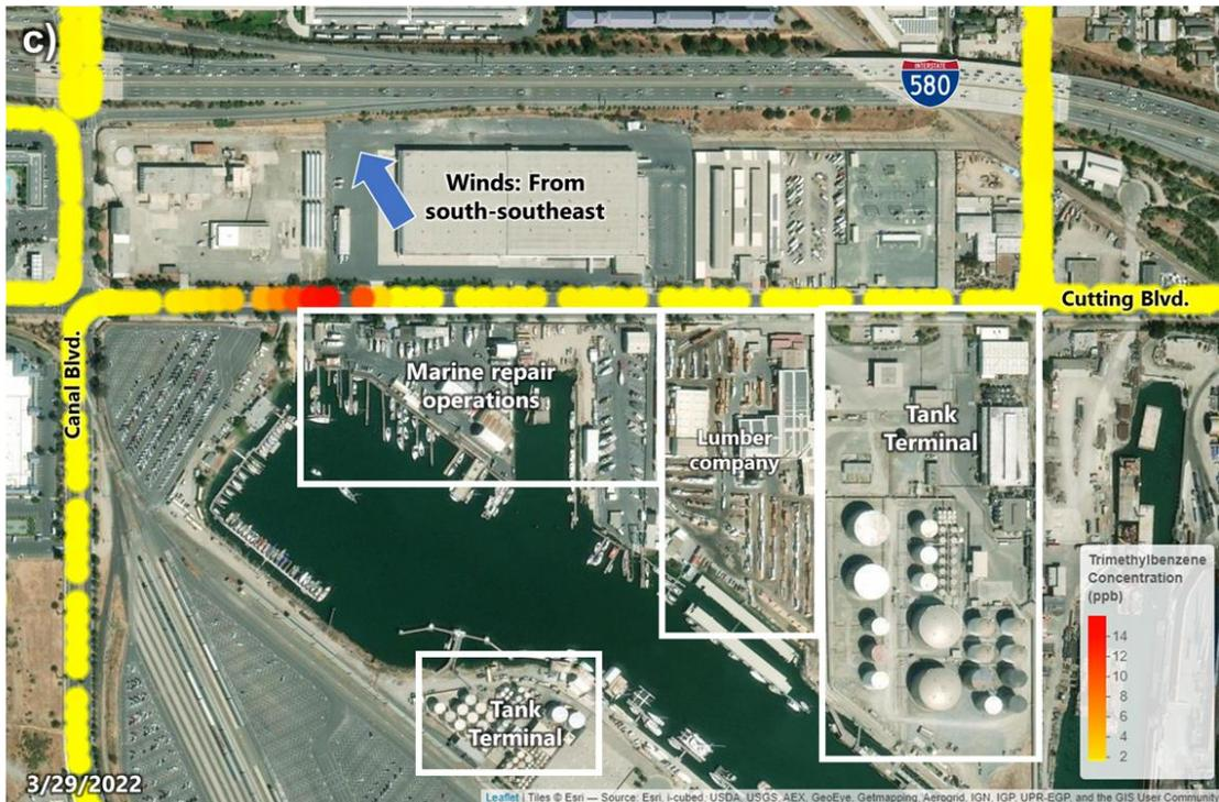
Figures 7b and 7c. Map views of trimethylbenzene concentrations measured along Cutting Boulevard near tank terminals and marine operations on b) 3/16/2022 and c) 3/29/2022.
