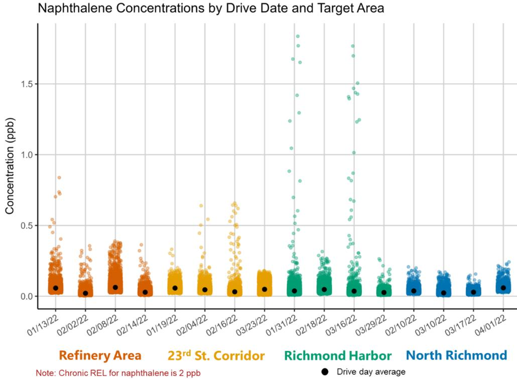
**Figure A-9.** Instantaneous (1-second) naphthalene concentrations by drive date and target area. The chronic REL for naphthalene is provided for reference but note that the chronic REL is based on annual exposures.
