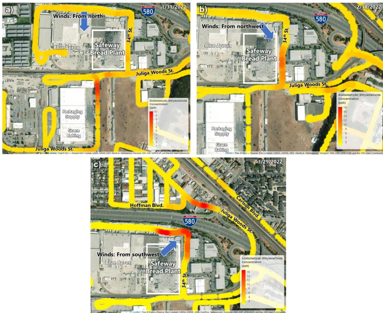
**Figure 17.** Map views of acetaldehyde + ethylene oxide concentrations measured in the vicinity of the Safeway Bread Plant on a) 1/31/2022, b) 2/18/2022, and c) 3/29/2022.
