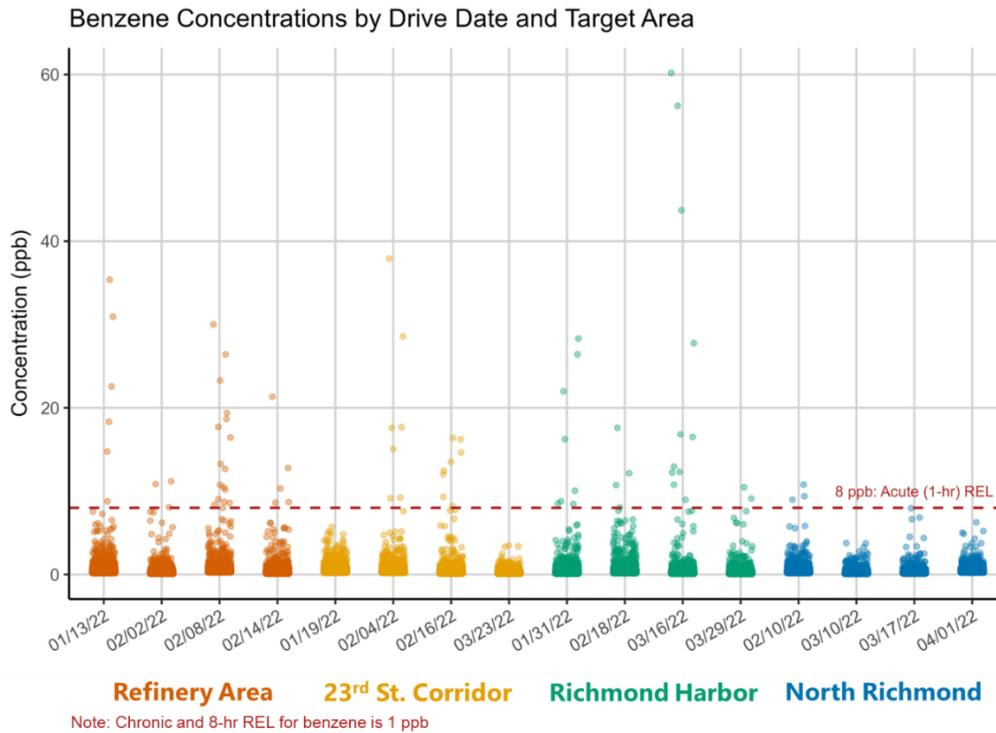
**Figure A-2.** Instantaneous (1-second) benzene concentrations by drive date and target area. The acute REL for benzene is provided for reference but note that the acute REL is based on 1-hour exposures.
