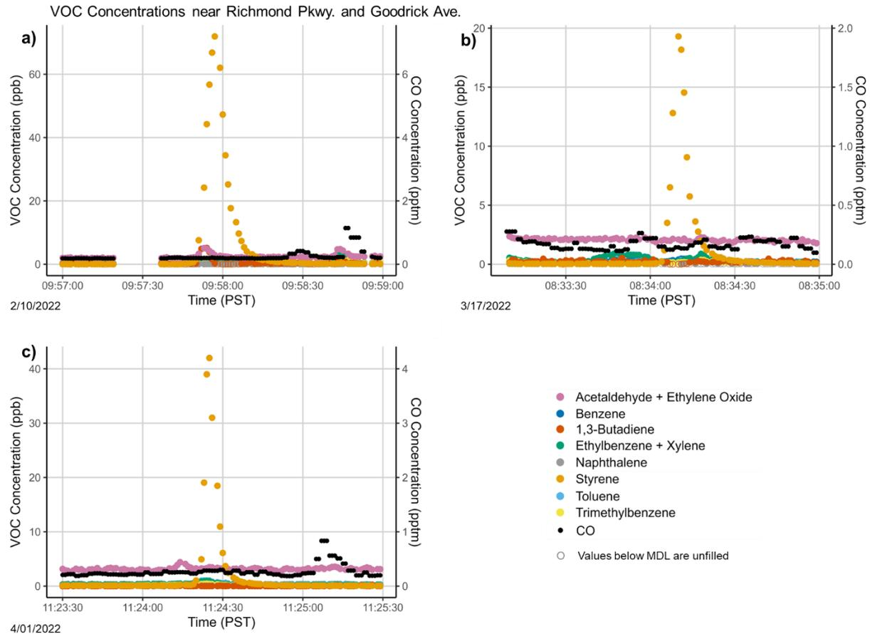
**Figure 10.** Time-series of VOC and CO concentrations measured along Richmond Parkway and Goodrick Avenue near a plastics fabrication facility on a) 2/10/2022, b) 3/17/2022, and c) 4/01/2022.
