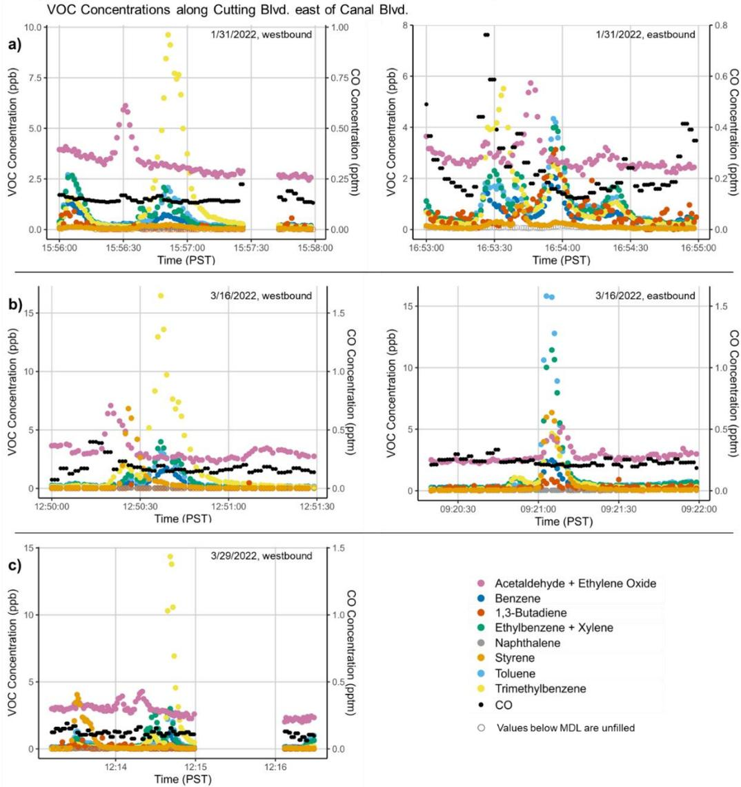
**Figure 8.** Time-series of VOC and CO concentrations along Cutting Boulevard measured near tank terminals and marine operations on a) 1/31/2022, b) 3/16/2022, and c) 3/29/2022.
