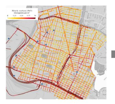
**Data**: 3 million air pollution measurements using fast response sensors on Google Street View cars over 1 year. Mapped at 30m resolution.
