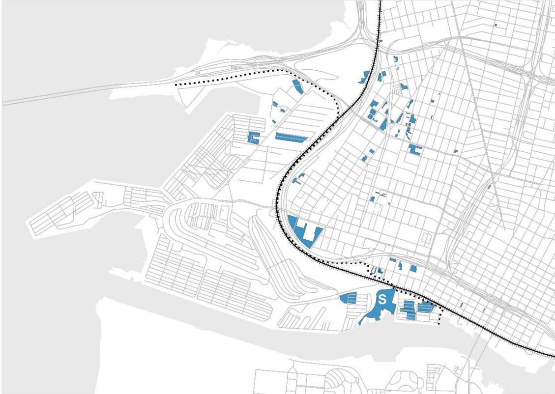
**Figure 3-8.** Area source polygons used to model emissions from truck-related businesses. The “S” indicates the location of Schnitzer Steel.
