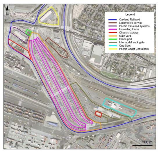
**Figure 6-1.** Layout of operations at the UP railyard in West Oakland. The components delineated represent different emissions sources (obtained from Gary Rubenstein, personal communication, 5 April, 2019).
