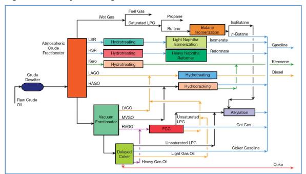
Figure 1: Refinery Flow Diagram
