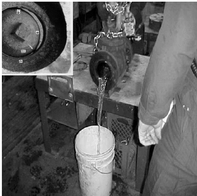
Figure 7. Leak test of the naphtha stripper level control bypass valve (B) in the closed position, showing significant water flow.
