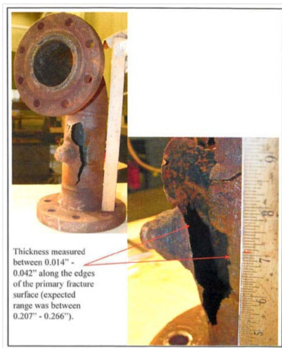
Figure 13. Failed piping component that resulted in the 2007 Richmond crude unit fire. This carbon steel piping was found to contain less than 0.005 percent silicon.
