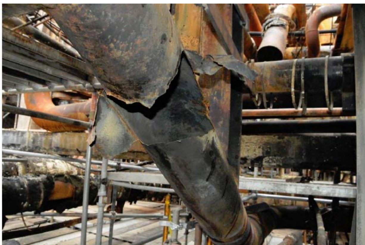
Figure 7. Photo of rupture on 4-sidecut 52-inch component.
