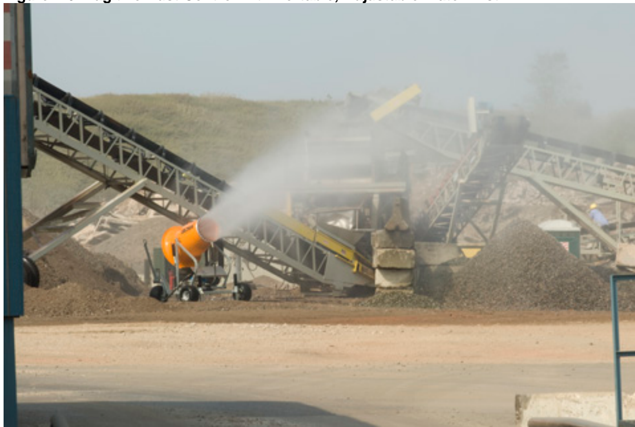
Figure II-6: Fugitive Dust Control with Portable, Adjustable Water Mist
