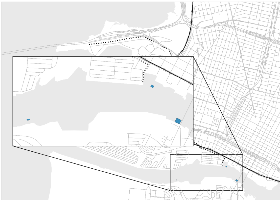
Figure 3-18. Area source polygons used to model emissions from ferries and excursion vessels at berths.
