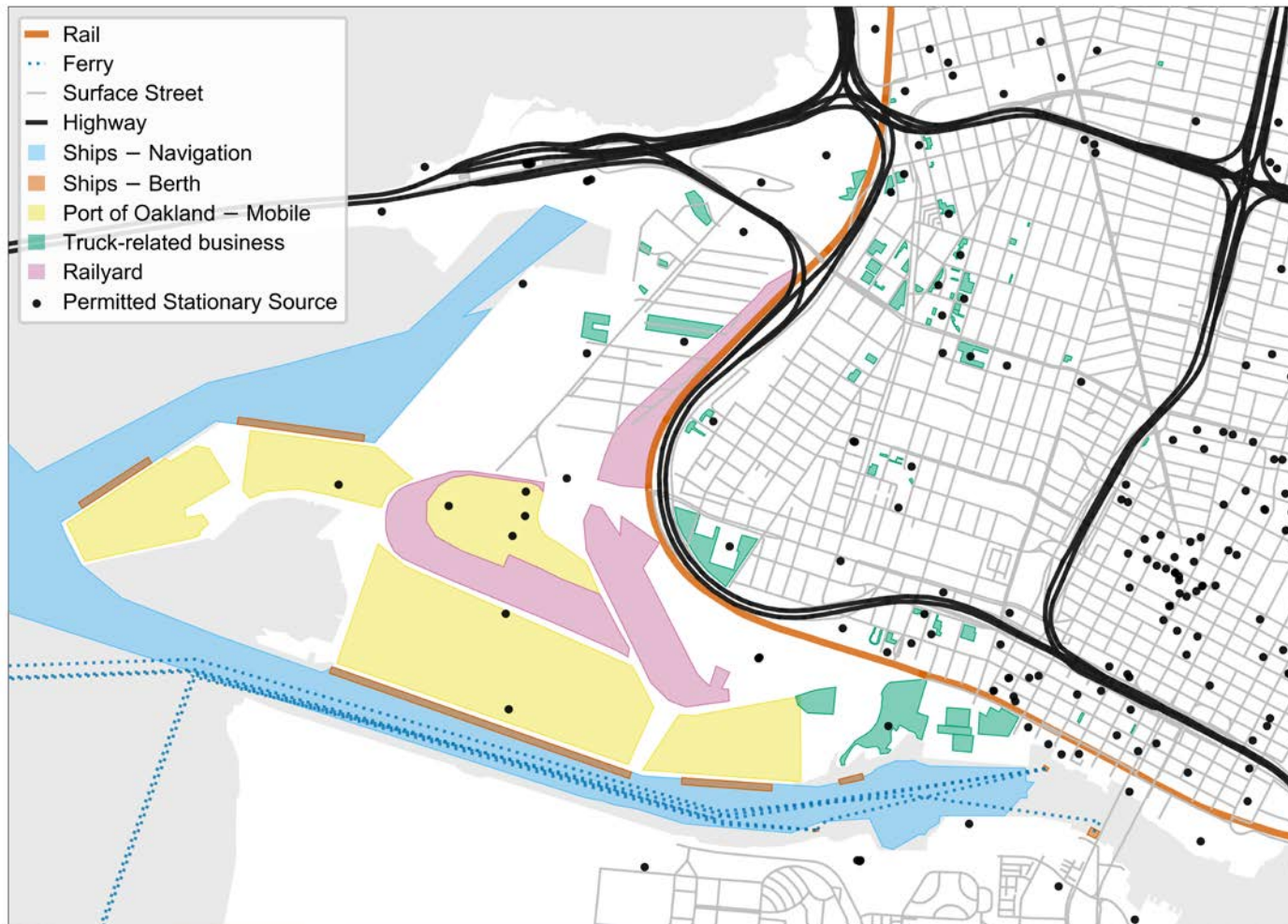
Figure 2-2. Composite of emissions source categories locations for the community-scale modeling in West Oakland. Ships – Navigation encompasses the areas of emissions from ocean-going vessels (maneuvering) and commercial harbor crafts (assist tugs, dredgers, and bunkering tugs and pumps) at the Port, as well as ships transiting to Schnitzer Steel; Ships – Berth includes berthing areas for ships at the Port, Schnitzer Steel, commuter ferries, and excursion vessels. Port of Oakland – Mobile encompasses the areas of emissions from Port Truck activity (idling and transiting) and cargo-handling equipment; Surface Street may include on- and off-ramps. Only permitted stationary sources that were modeled are included.
