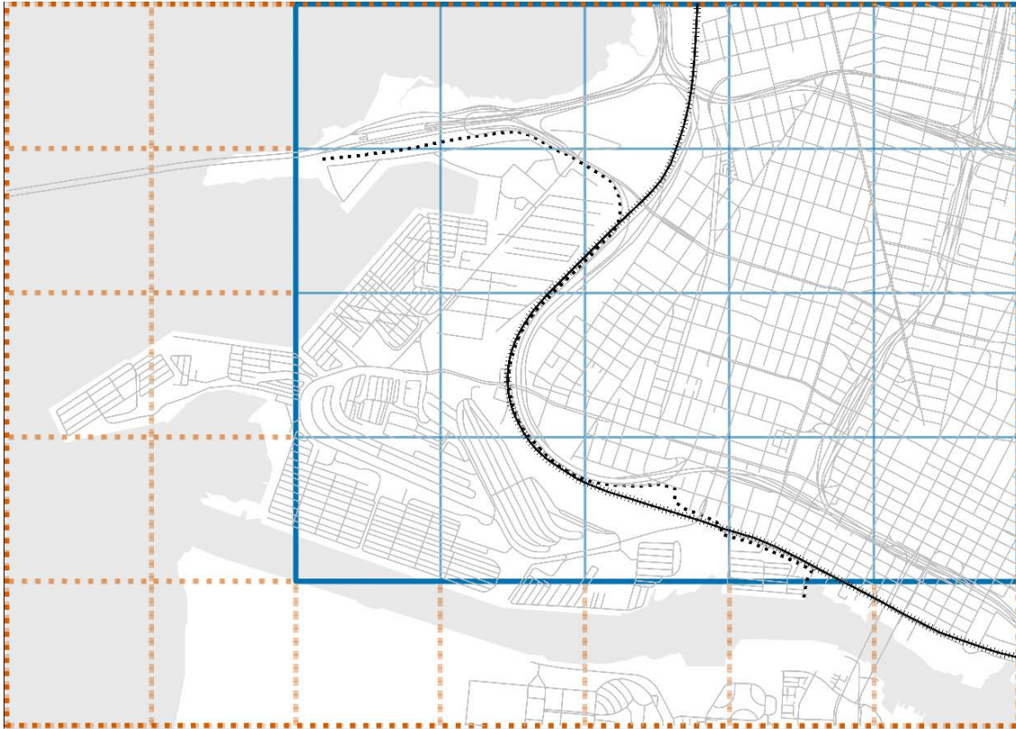
Figure 3-3. Extents of the Source Domain (red dotted lines) and Receptor Domain (blue solid lines) used in AERMOD modeling. The inner tiles represent the 1 km × 1 km grid cells of the regional modeling.
