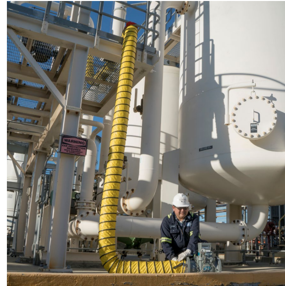
Measuring emissions from a stack from a pollution control device
