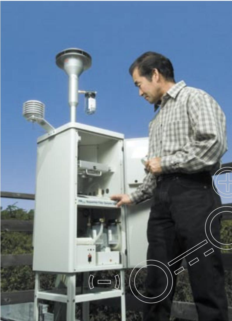
A SUPERVISOR IN THE AIR DISTRICT'S AIR MONITORING SECTION, STAN CHANGES A FILTER ON A PM<sub>2.5</sub> SAMPLER AT THE SAN FRANCISCO MONITORING STATION. AIR MONITORING STATIONS TELL US IF THE BAY AREA IS MEETING AIR QUALITY STANDARDS AND PROVIDE DATA FOR DAILY AIR POLLUTION FORECASTS AND MODELING.
