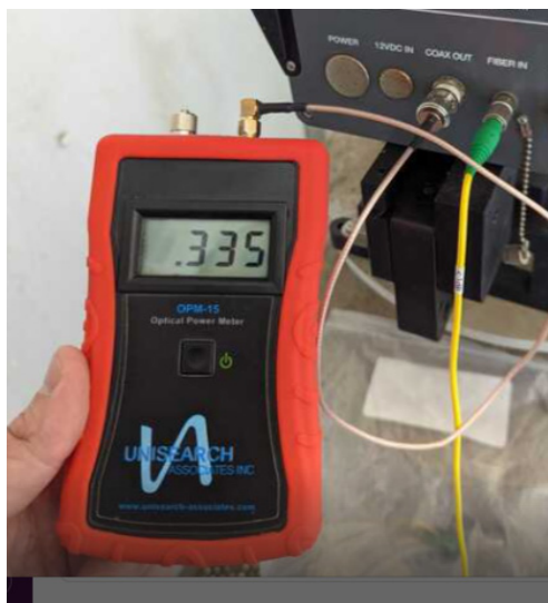
Figure D5. Measuring laser power with the OPM 15 meter provided.
