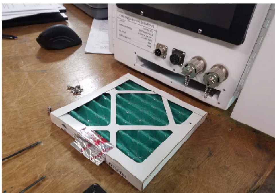
Figure A-7. Filter completely removed.
