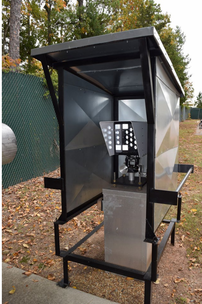
Figure 13. A UV-DOAS retroreflector.
