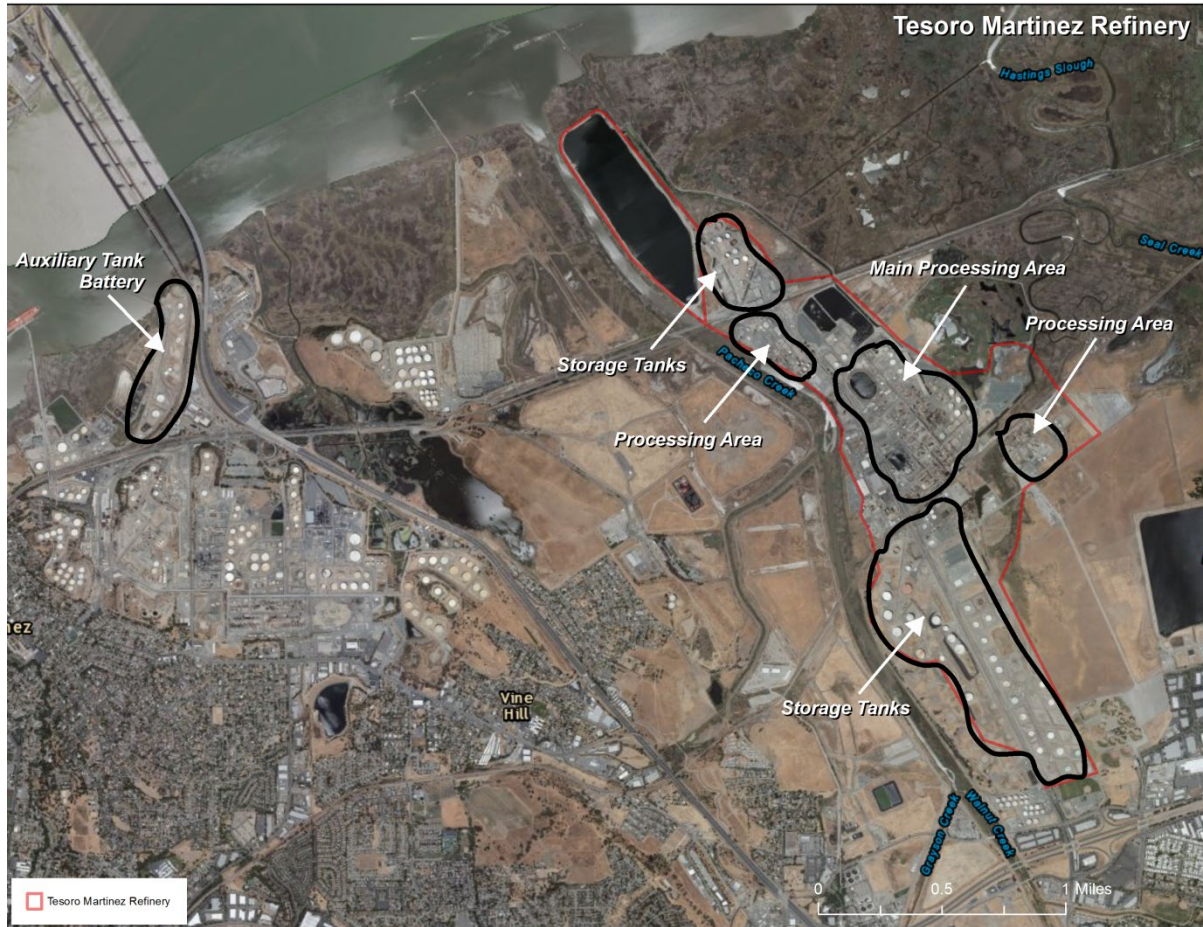
Figure 4. Layout of the Martinez Facility.
