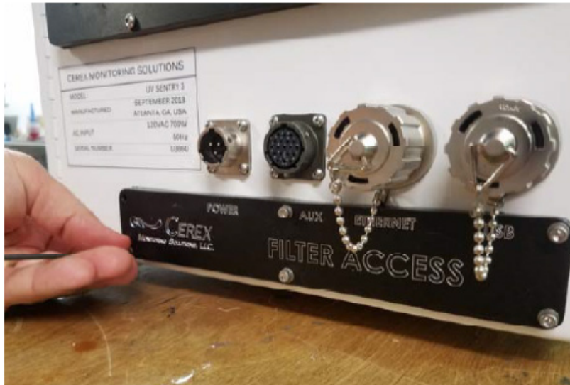
Figure A-5. Location of filter access plate.
