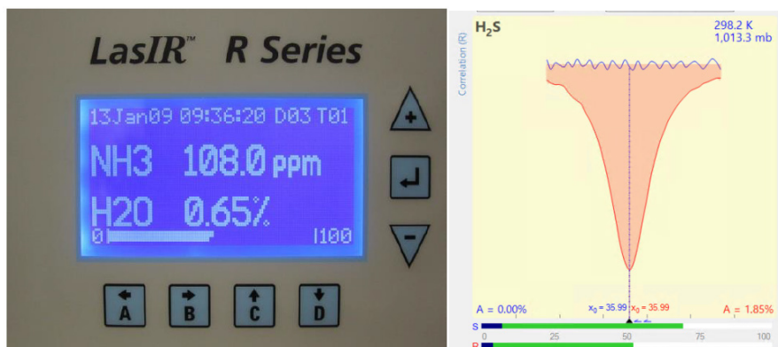
Figure D-4. Main running window on instrument front panel (left) and scope display in LasIR View software (right).
