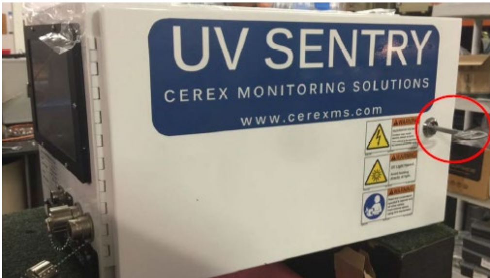
Figure 9. Opening the source access panel.
