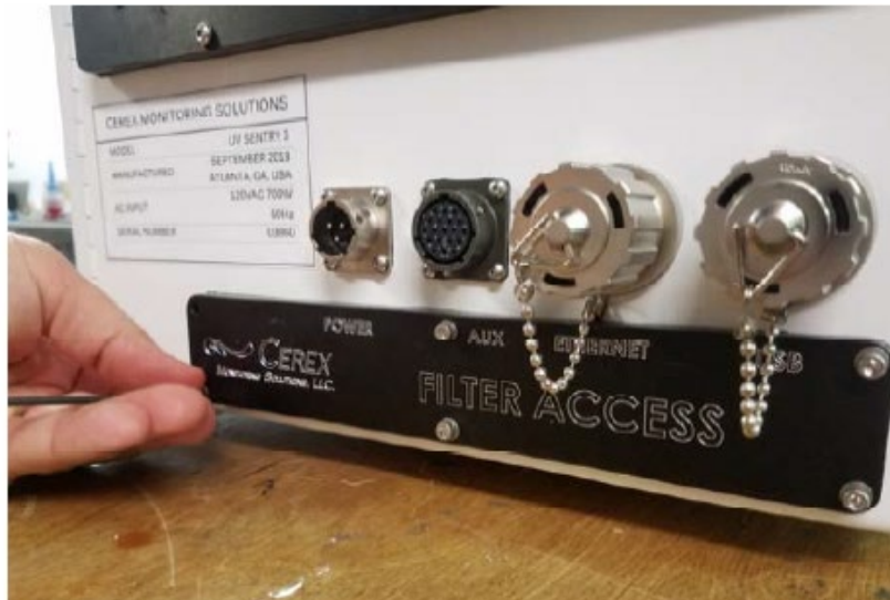
Figure 5. Location of filter access plate.
