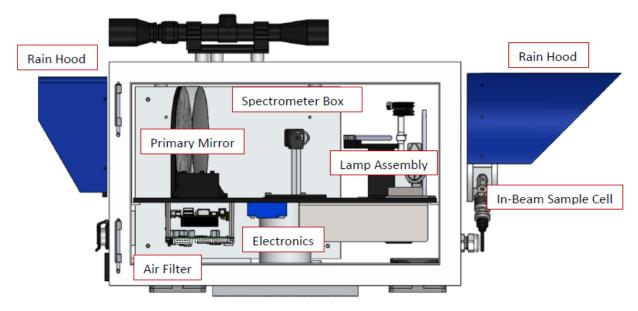
Figure 1. Schematic of the monostatic UV Sentry UV-DOAS analyzer.
