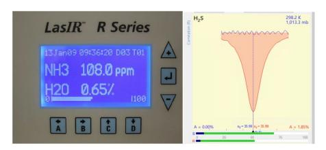
**Figure 4.** Main running window on instrument front panel (left) and scope display in LasIR View software (right).
