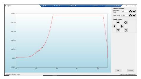
**Figure 4.** An example of a saturated spectrum when in **Align** mode. Note the "flat top" profile of the spectrum. The spectrum flattens out because the detector has saturated at those wavelengths and cannot quantitatively measure additional light.
