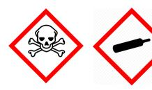
WARNING – Toxic Gas and Eye Hazard. H<sub>2</sub>S is a highly toxic gas that can cause death and other adverse health effects at concentrations above 100 ppm. This procedure requires the use of concentrations as high as 750 ppm H<sub>2</sub>S for the span check. This procedure must be conducted in a well-ventilated area and requires gas monitors, respirators, and the use of fume scrubbers. Make sure you and others fully understand
