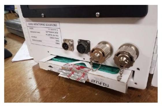
Figure 6. Filter access plate removed and filter partially removed.
