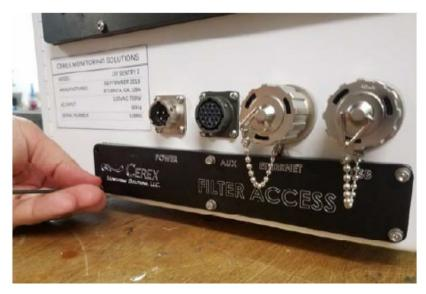
Figure 5. Location of filter access plate.
