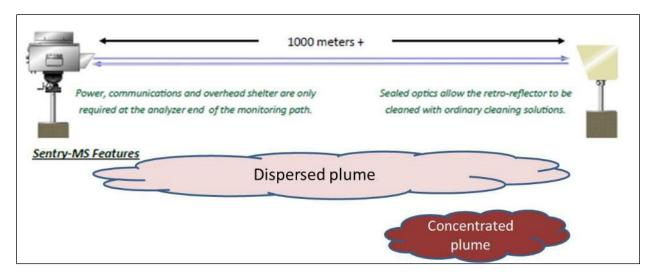
**Figure 16**. Basic premise for open-path instrument operation. Image from Cerex Sentry-MS monitoring brochure, used with permission from Cerex Monitoring Solutions, LLC.
