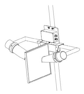
Figure 2. Scatter plate mounting.
