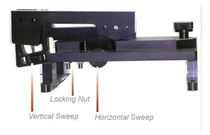
Figure 2. Location of adjustment knobs used for alignment of the Unisearch TDLAS.
