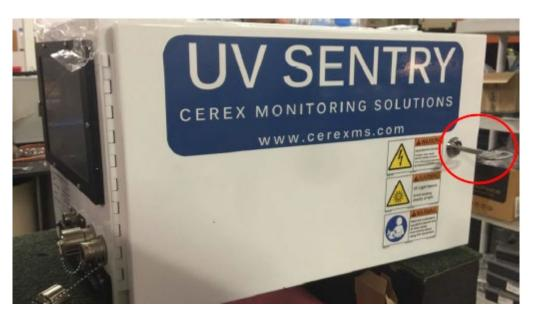
Figure 9. Opening the source access panel.
