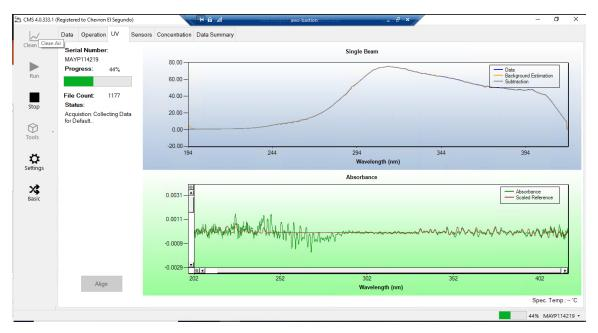
**Figure 2.** Screenshot showing the **UV** tab of the CMS software. Note that the **Align** button is grayed out because the instrument is in run mode (the **Run** button is also grayed out because the instrument is in run mode).
