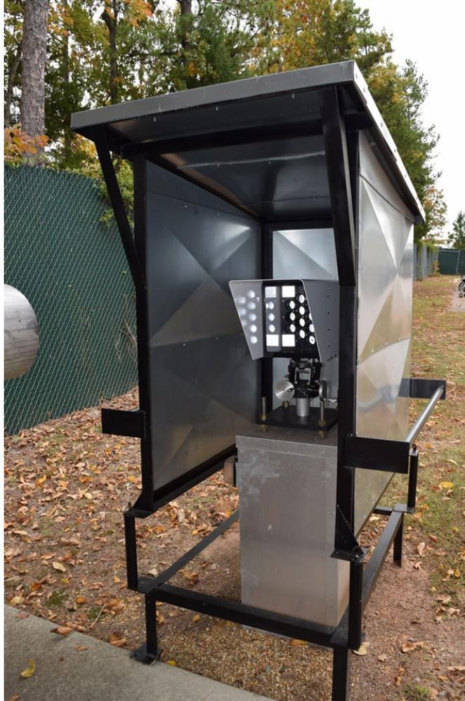
**Figure 18.** Example of a UV-DOAS retroreflector installation.
