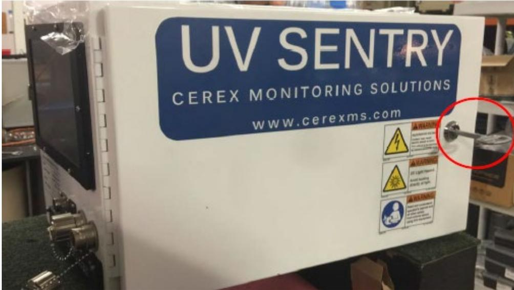
Figure 9. Opening the source access panel.
