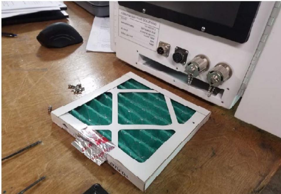
Figure 7. Filter completely removed.
