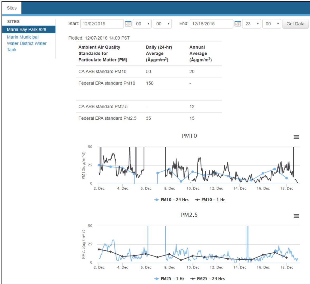
Figure 20. Example of non-public field operations website used for daily review of instrument operations.
