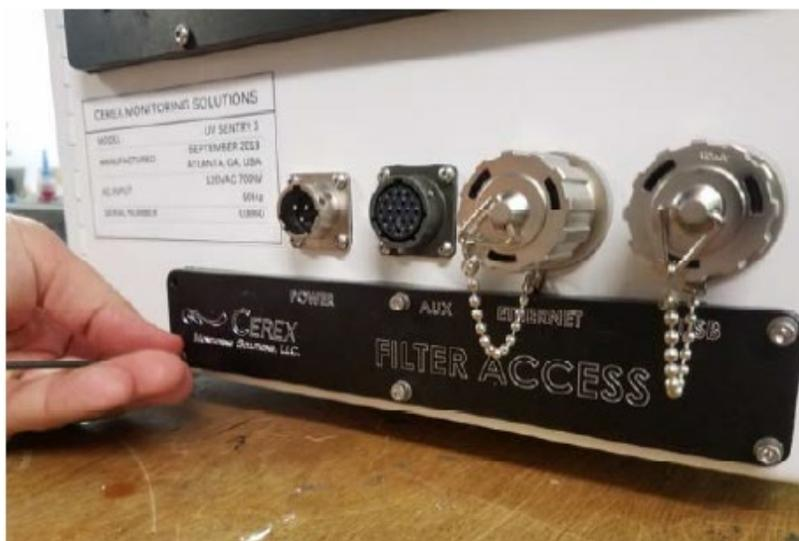
Figure 5. Location of filter access plate.
