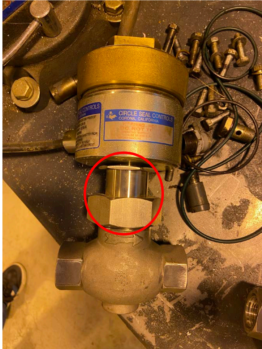
Figure 2: Fully assembled 6210 valve. The plunger that is known to unthread itself is located within the valve body circled in red.
