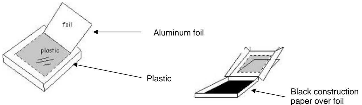
3. Cut another piece of aluminum foil to line the bottom of the pizza box and carefully glue into place. Next, cover the aluminum foil in the bottom of the pizza box with a piece of black construction paper and tape into place.
