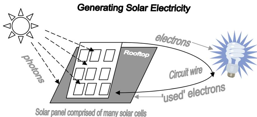
1. Explain to the class that they will be learning how a solar cell generates electricity. Draw a solar panel on the chalkboard following the steps below. Use the above diagram to guide you. Engage students as you draw each component to ensure comprehension:
