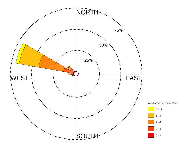
Windrose depicting distribution of wind direction and speed at Bethel Island during summer 2016 (Jun 1 - Aug 31). Length of each 20 degree wedge indicates the percentage of time inflow winds are from the indicated direction. The color scale denotes wind speed intensities (in meters per second).
