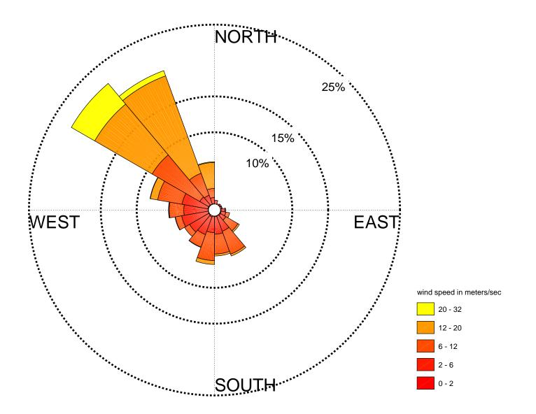
Windrose depicting distribution of wind direction and speed at Bodega Bay during summer 2016 (Jun 1 - Aug 31). Length of each 20 degree wedge indicates the percentage of time inflow winds are from the indicated direction. The color scale denotes wind speed intensities (in meters per second). Source: BAAQMD 2016
