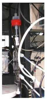
Photos of the inlet duct and fan control, stainless steel plenum exiting duct, and glass plenum with particle filter (replaceable paper disk filter is in the orange cartridge).
