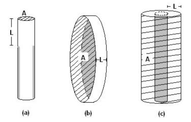
Figure 0-8. Schematics of (a) tube, (b) shield, and (c) radial geometry passive samplers with path length, L; Dashed area represents diffusive path area, A; Grey area represents adsorbent surface.
