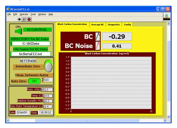
Initial screen view of photoacoustic instrument LabView program
