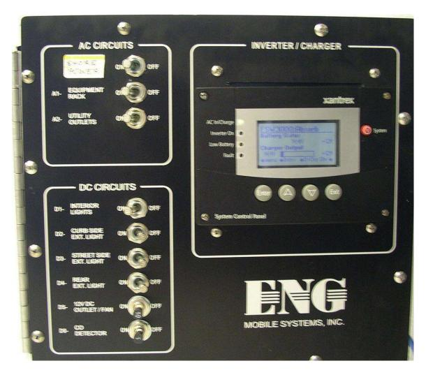
When operating the equipment with the van connected to an external AC line (aka "shore power"), the toggle switches in the upper left section should be in the ON position, as shown above. If starting up without shore power, flip on AC Circuit switches for inverter, instrument rack, and utility outlets after starting the inverter, as described below.
