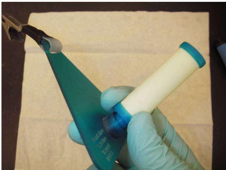
Assembly of the Radiello Passive Sampler is now complete. Use the metal clip to attach the sampler to clothing for personal exposure monitoring or to another object for ambient monitoring.
