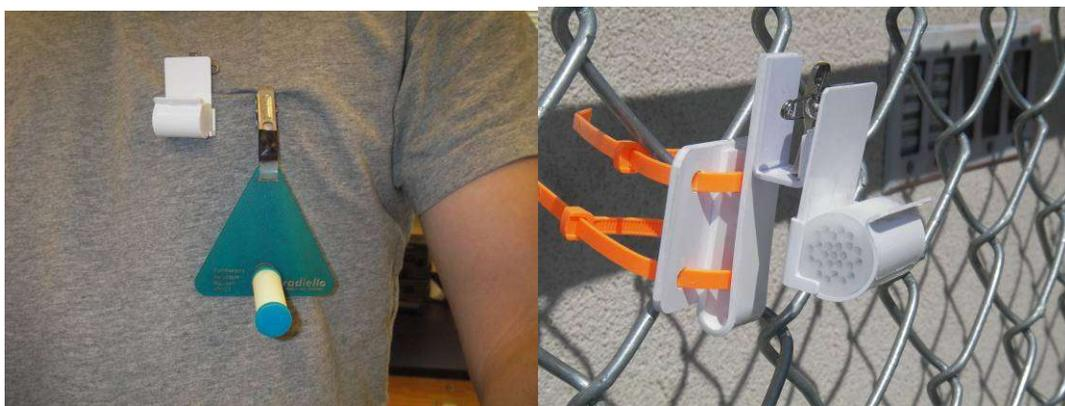
The *Mounting Bracket* can be easily attached to objects such as fences and poles with zip ties. If sampling outdoors, the *Opaque Vial* should be used as a shelter. It can easily be slipped over the *Mounting Bracket* and sampler as shown below. Keep the *Opaque Vial* lid and sealed *Sample Bag* for later. Note time and date when sampling begins.
