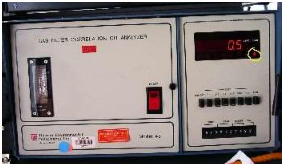
TEI CO analyzer front panel with light indicating instrument is in Span mode circled – this indicator should be off when collecting data.
