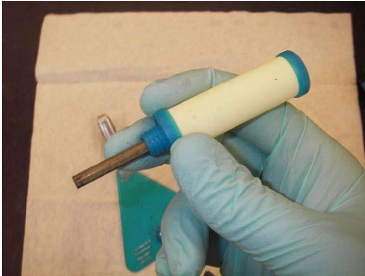
Next, screw the *Diffusive Body* into the *Supporting Plate* as shown below. Be careful, to ensure the threads are aligned properly before tightening. The fit should be snug, but do not over-tighten as this can result in breaking the *Supporting Plate* or the *Diffusive body*. Screw the assembly together upside-down to ensure that the *Adsorbing Cartridge* is not protruding from the end of the *Diffusive Body* during tightening.
