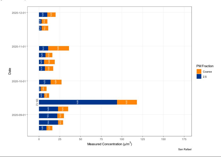
Figure J.4 - Comparison of Fine and Coarse Fractions of 24-Hour PM<sub>10</sub> Measurements at the San Rafael Station (8/16/2020 - 11/30/2020)
