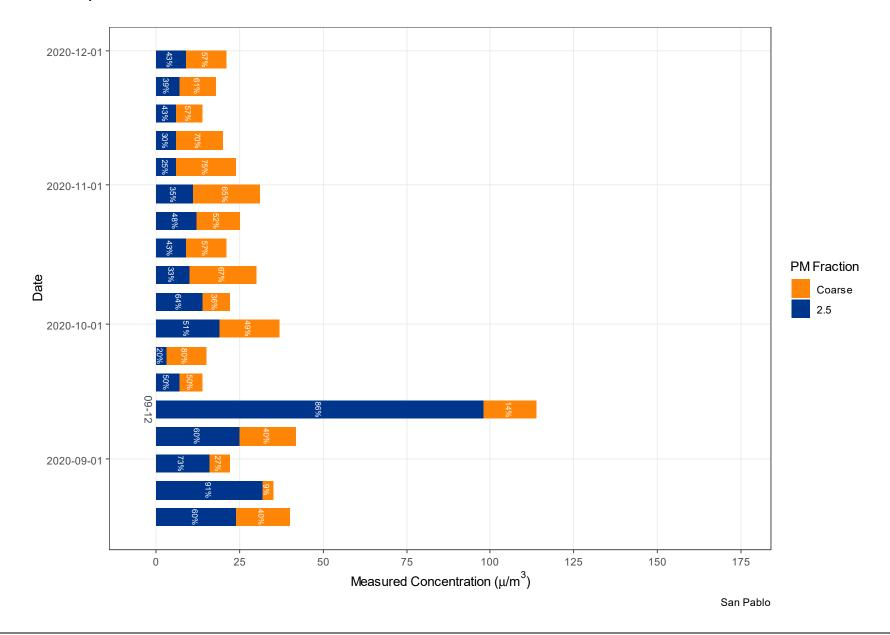
Figure J.3 - Comparison of Fine and Coarse Fractions of 24-Hour PM<sub>10</sub> Measurements at the San Pablo Station (8/16/2020 - 11/30/2020)
