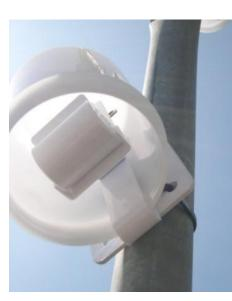
Ogawa passive samplers for  $NO_2/NOx$  and  $SO_2$ (thumb size in cup shield)
