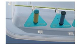
Radiello passive samplers for VOC, aldehydes and  $H_2S$  (size of a roll of pennies)
