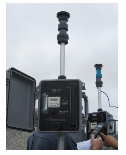
AirMetrics Minivol Aerosol Sampler (10" diameter x 24" tall) 12V battery or 110VAC
