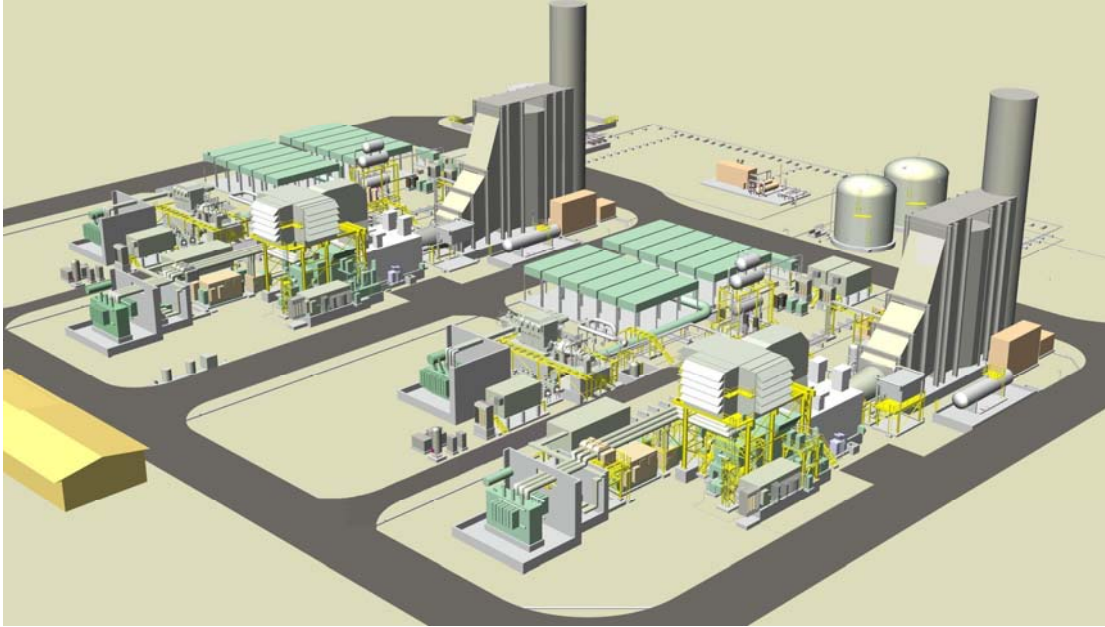
Figure 8: 3-D Model of Two-Unit SCC6-5000F 1x1 Flex-Plant™ 10
